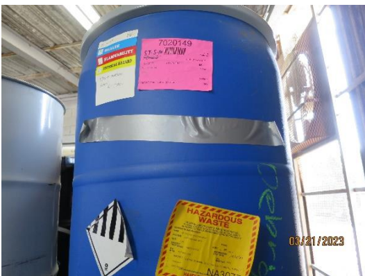
Photo #5 - Container missing an indication of the hazards.
