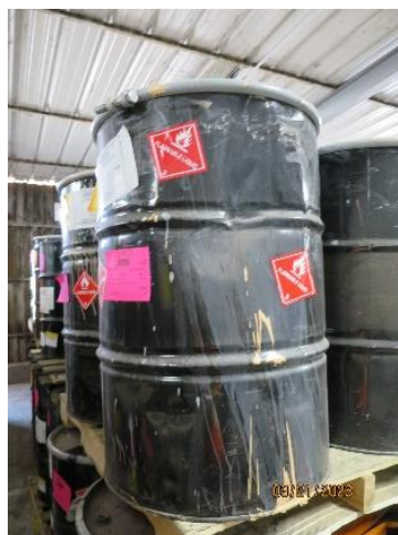
Photo #8 - A 55-gallon damaged container.
