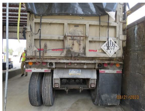
Photo #30 – Missing an indication of the hazards of the contents.
