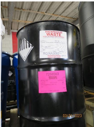
Photo #3 – Container missing an indication of the hazards.
