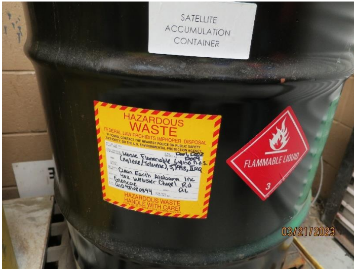
Photo #49 – 30-gallon waste container accumulating liquid hazardous wastes in the lab storage room.
