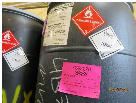
Photo #46 – Pharmaceutical wastes not identified with an appropriate EPA hazardous waste code.
