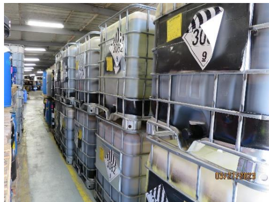
Photo # 6 – Containers missing an indication of the hazards.
