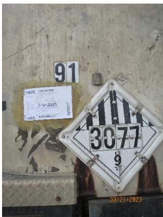
Photo #29 – Missing an indication of the hazards of the contents.
