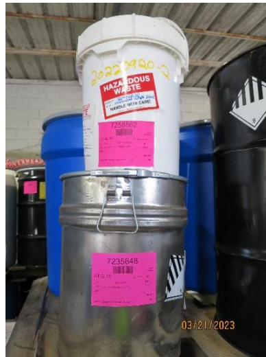
Photo #4 – Containers missing an indication of the hazards.
