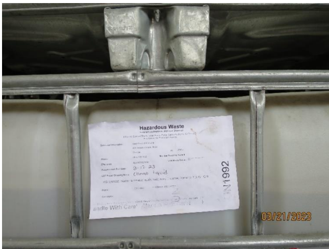
Photo #27 – Pharmaceutical waste tote missing applicable P waste codes.
