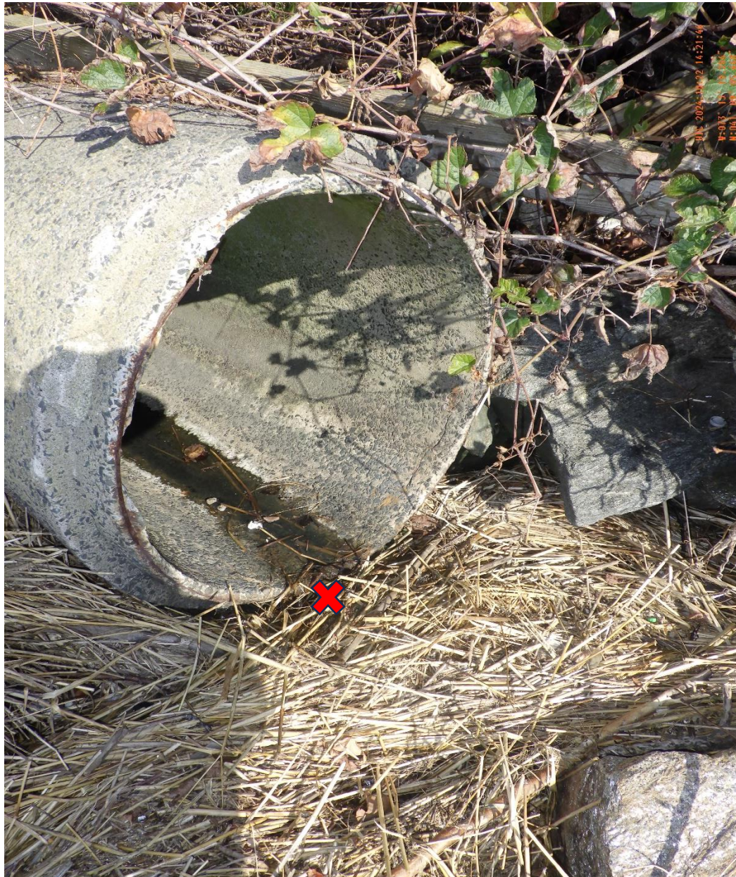
Photo 2: Beacon1 (photo taken 10/22/2024 at approx. 10:21 Outfall located near 2 Seabright Ave, discharging into the Long Island Sound. Sample point is indicated by a red X. (Note1: Time stamp on photo is incorrect) (Note 2: Not enough flow to collect adequate sample volume for PCP, enterococcus analysis, conductivity, salinity, and temperature. Only enough discharge to analyze for ammonia, surfactants, and total chlorine.)
