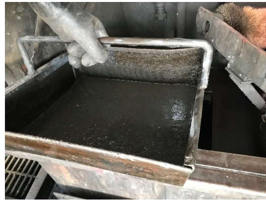
Picture 5: Hazardous Waste Sludge and Debris in the Tray, Return and Fill Area (D001, D006, D008, D018, D039 and D040)
