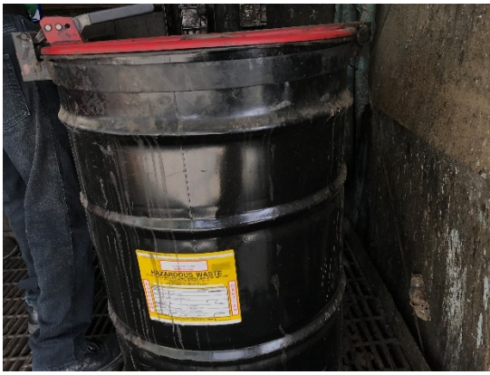
Picture 7: 55-gallon SAA Drum in the Return and Fill Station
