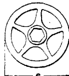
Style E Wheel , Malleable Iron Round Pattern, Oval Rim, Hexagon Hole
