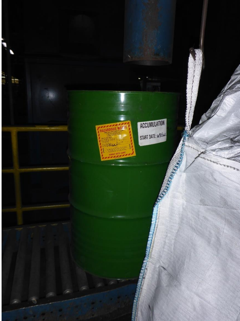
Photo 3: 55-gallon drum behind supersack shown in Photo 1. Drum is positioned under the other bleed-out chute and contains mold sand that was discharged from the storage tank so that the tank could be replenished with new sand. The drum has no lid. It is labeled D008 hazardous waste solid contains copper, lead and zinc, and marked with an accumulation start date of 02/09/2021.
