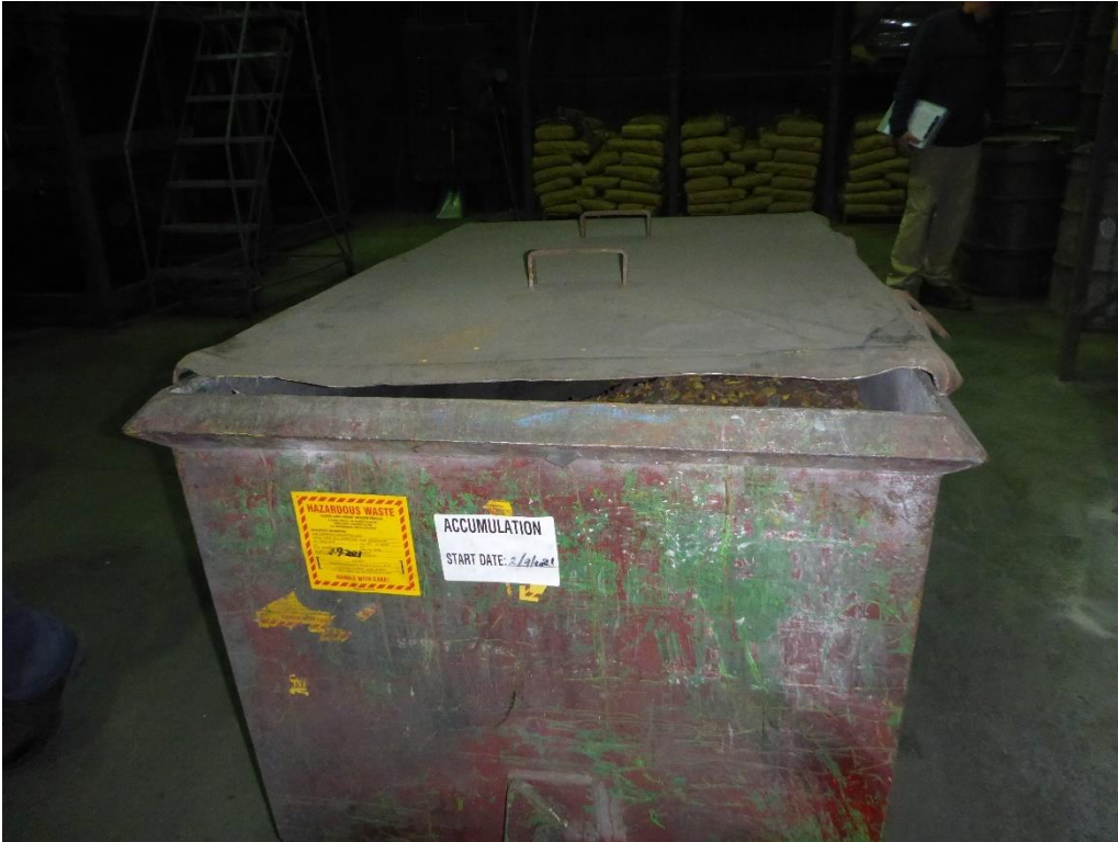
Photo 8: One hopper of on the floor in the middle of the Reclaim Room. Hopper was labeled as D008 hazardous waste containing copper, lead and zinc. It was dated 02/09/2021. The hopper appeared to contain cores and core sand for processing in the Reclaim Room. Shot blast that is recovered in the Reclaim Room is reused on-site in the Wheelabrator; metals that are recovered in the Reclaim Room are remelted and reused in the casting process; foundry sand that is segregated in the Reclaim Room is disposed of as D008 hazardous waste.
