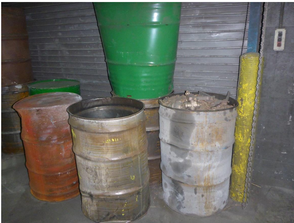
Photo 17: 55-gallon drums in the Reclaim Room. No labels, and could not determine if contents will be processed here or have already been processed.
