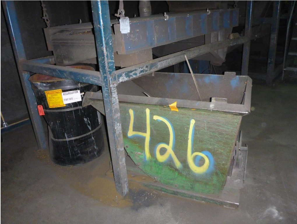
Photo 11: Metal hopper and 55-gallon drum for accumulating separated material that has been processed in the Reclaim Room. The hopper is labeled D008 hazardous waste 02/08/2021 and appears to contain used foundry sand. The 55-gallon drum is labeled D008 hazardous waste 02/08/2021 and appears to contain metal shavings.
