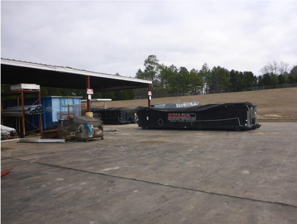
Photo 34: Two roll-off containers used to store and ship supersacks of D008 hazardous waste baghouse dust. One roll-off staged and open to receive supersacks, and the other stored under the metal roof. Both containers were labeled D008 hazardous waste solid (contains copper, lead and zinc) and identified with the UN3077. The open container was dated 02/09/2021, and the closed container was dated 02/08/2021.
