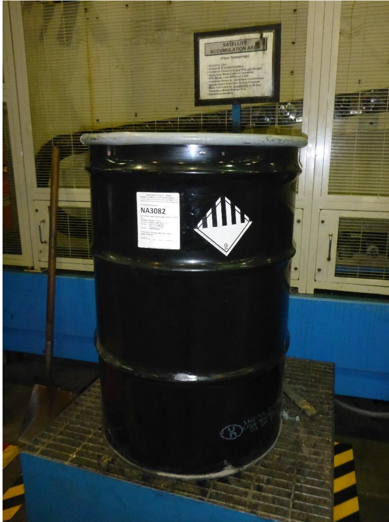
Photo 21: SAA for accumulating floor sweepings generated in part of the Machining area. 55-gallon drum labeled D008 hazardous waste liquid (lead shavings, oil/grease and water) and identified with a DOT class 9 hazard placard. Ring was not secured on the drum, so Mr. Peebles closed the drum by securing the lid with the ring.
