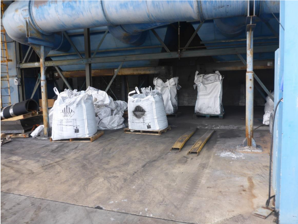
Photo 32: Two supersacks observed connected to the Sand System Baghouse. Bags are not closed, labeled as hazardous waste, or marked with an accumulation start date.
