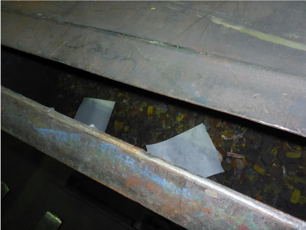
Photo 9: Close up of contents in hopper observed on the floor in the middle of the Reclaim Room shown in Photo 8. Hopper was labeled as D008 hazardous waste containing copper, lead and zinc. It was dated 02/09/2021. The hopper appeared to contain cores and core sand for processing in the Reclaim Room. Shot blast that is recovered in the Reclaim Room is reused on-site in the Wheelabrator; metals that are recovered in the Reclaim Room are remelted and reused in the casting process; foundry sand that is segregated in the Reclaim Room is disposed of as D008 hazardous waste.
