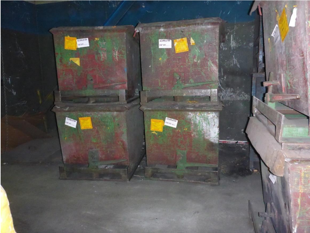
Photo 15: Metal hoppers near the door in the Reclaim Room. This area contained a total of ten metal hoppers. Eight of the hoppers were empty, and all were labeled D008 hazardous waste and marked with an accumulation start date. The oldest hopper was dated 02/01/2021. Personnel did not know if the hoppers contained material ready for reclamation or material that had already gone through the separation process.
