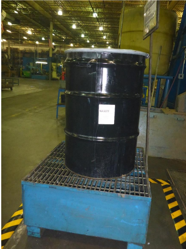
Photo 23: SAA for accumulating floor sweepings generated in part of the Machining area. 55-gallon drum labeled D008 hazardous waste air filters. Personnel immediately relabeled as D008 hazardous waste contaminated debris.
