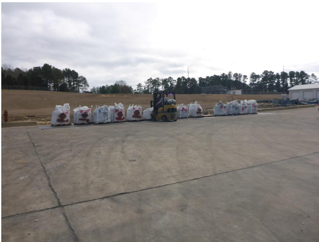
Photo 36: Supersacks of D008 hazardous waste baghouse dust staged on the scale for weighing before being placed into open roll-off container for storage and shipment.
