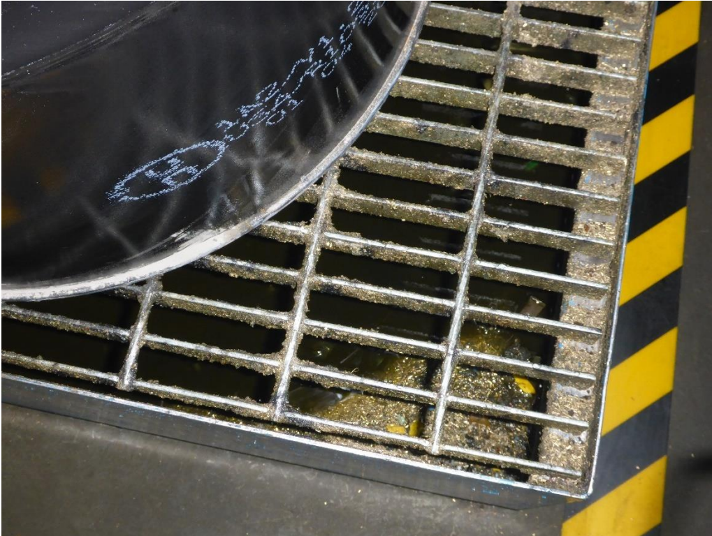
Photo 22: SAA for accumulating floor sweepings generated in part of the Machining area as D008 hazardous waste liquid (lead shavings, oil/grease and water). Material observed inside the secondary containment pallet.
