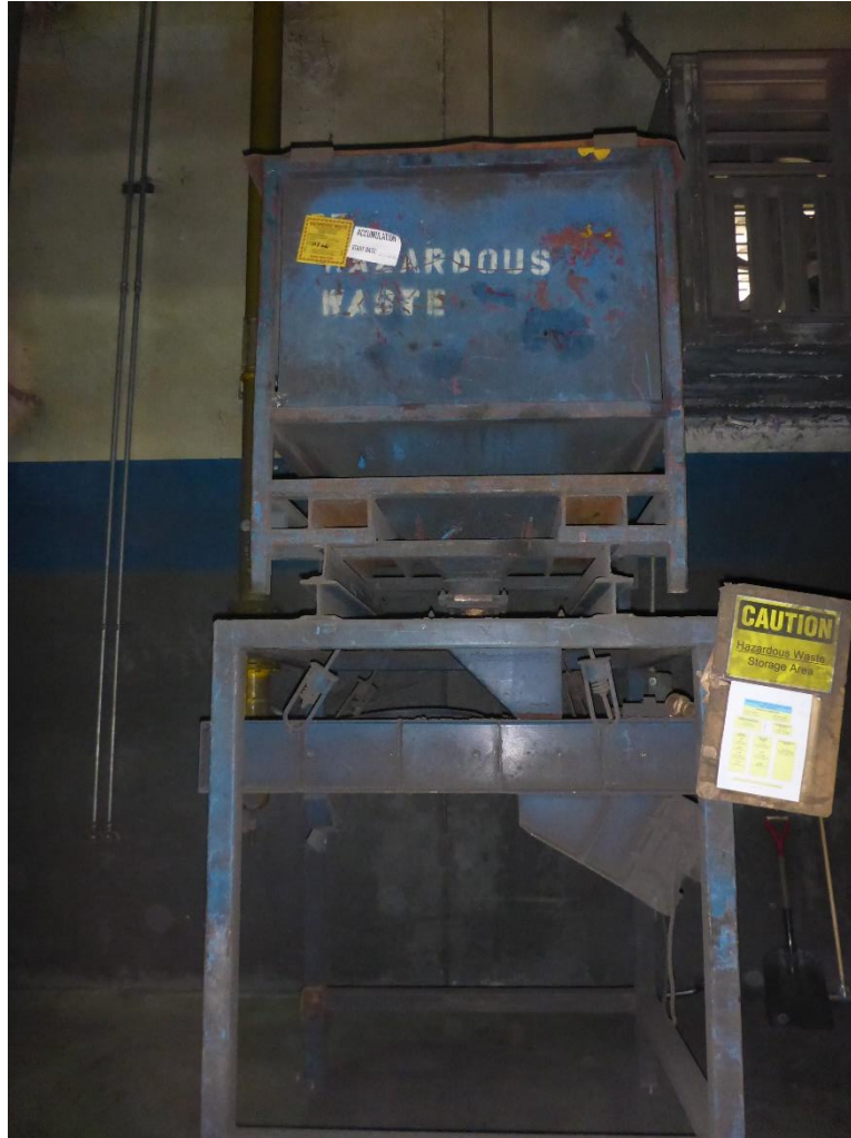
Photo 10: Metal hopper on elevated stand in the Reclaim Room. The hopper appears to be staged for processing. Shot blast that is recovered in the Reclaim Room is reused on-site in the Wheelabrator; metals that are recovered in the Reclaim Room are remelted and reused in the casting process; foundry sand that is segregated in the Reclaim Room is disposed of as D008 hazardous waste. The hopper was labeled as D008 hazardous waste containing copper, lead and zinc, and dated 12/08/2020.
