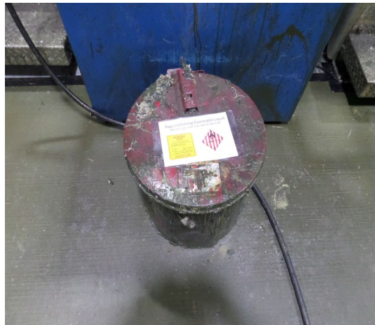
SAATI. Coating Line. Inspectors observed one 5-gallon empty container. The cover was not in good condition. Photograph 4 taken at 10:52 a.m.
