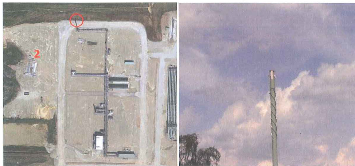
Figure 2. Emergency Flare. Left: Google map with a red circle indicating the location of the flare and a red number "2" indicating the location of the VISR instrument. Distance: 213 ft. Right: A photo of the flare taken during the test.
