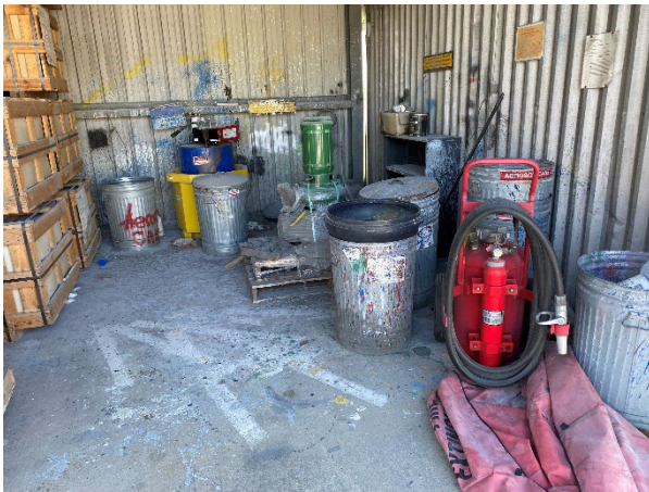
Photograph 2: Aerosol Can Piercing Station.
