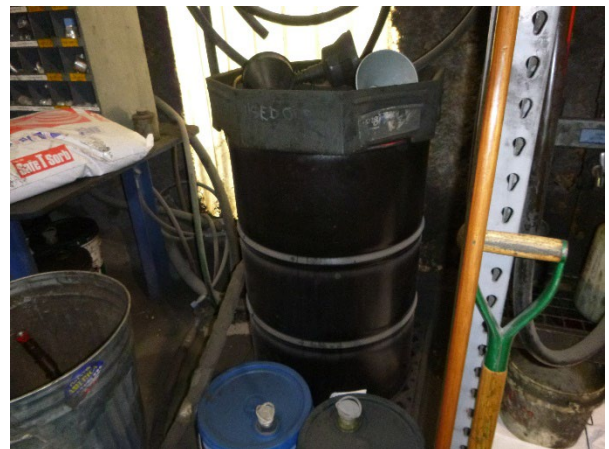
Photograph 32: Mobile Garage – container of used oil without Used Oil label.
