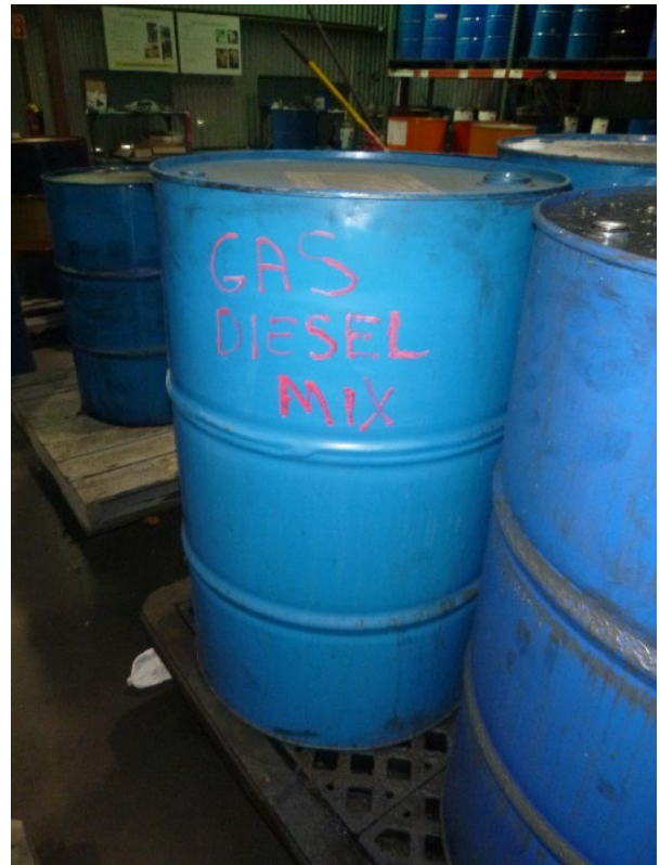
Photograph 4: Oil Building – Container without hazardous waste label and indication of the hazard.
