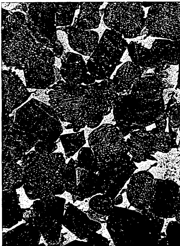
Fig. 2. Portland cement clinker. Gray oblong crystals are 3\text{CaO} \cdot \text{SiO}_2 , twinning structure is 2\text{CaO} \cdot \text{SiO}_2 , and the white interstitial material is 4\text{CaO} \cdot \text{Al}_2\text{O}_3 \cdot \text{Fe}_2\text{O}_3 in a matrix of darker glass. (Reflected light; \times 800 .)
