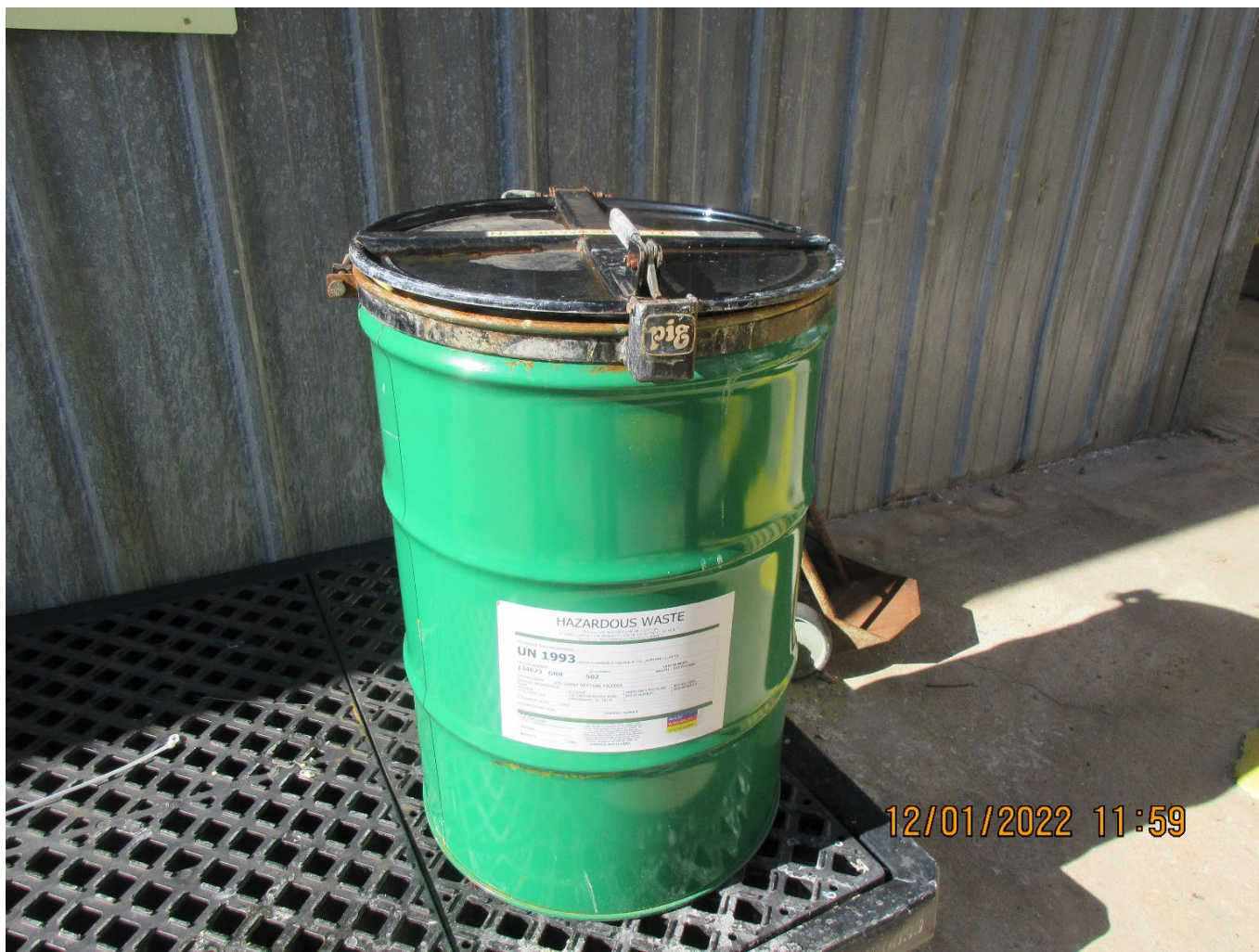
Photograph 12 – 55-gallon drum in SAA in South 330 Process Area collection of hazardous waste filters
