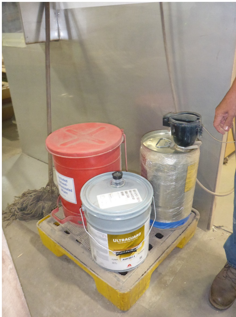
Photo 9: Wood Plant SAA for accumulating waste near the manual spraybooth. One red flip-top flammable can for accumulating excluded solvent contaminated wipes. One 10-gallon container of product material. 10-gallon container with latched funnel for accumulating D001 / F003 / F005 hazardous waste paint related materials.
