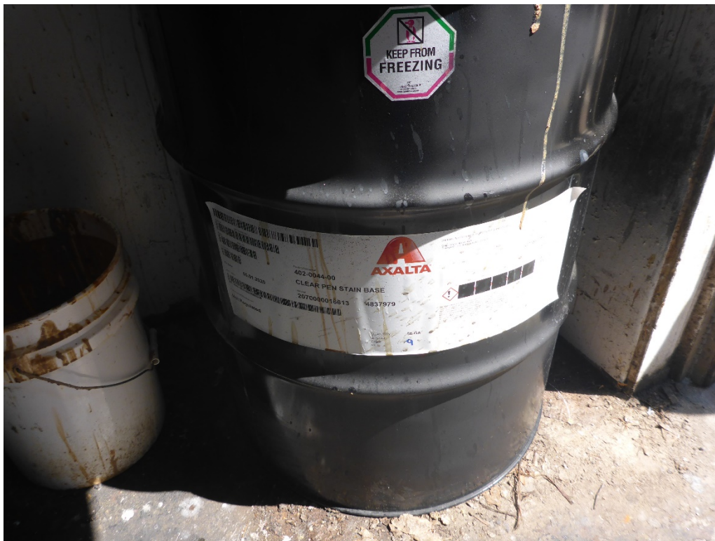
Photo 4: 55-gallon drum in the distillery SAA. Drum to be used for accumulating hazardous waste still bottoms, but it was not labeled with the words “hazardous waste” or with an indication of the hazards. Drum reported to be empty.
