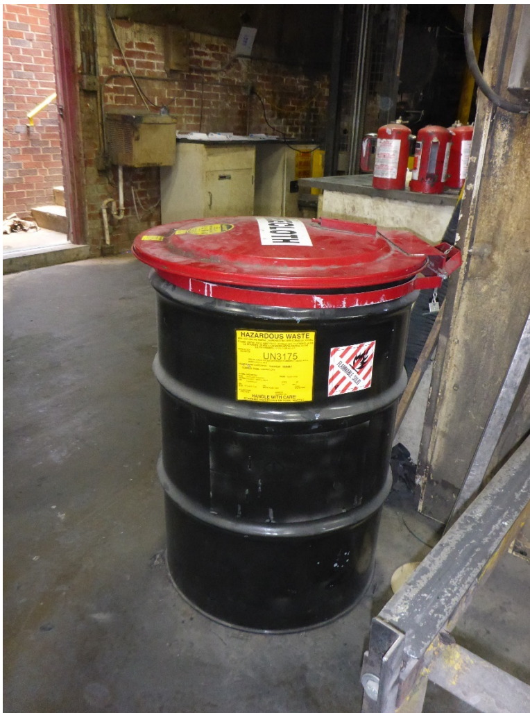
Photo 16: Resin Plant SAA for accumulating contaminated cheesecloth in the sinks area. 55-gallon drum with flip-top lid labeled D001 hazardous waste cheesecloth.
