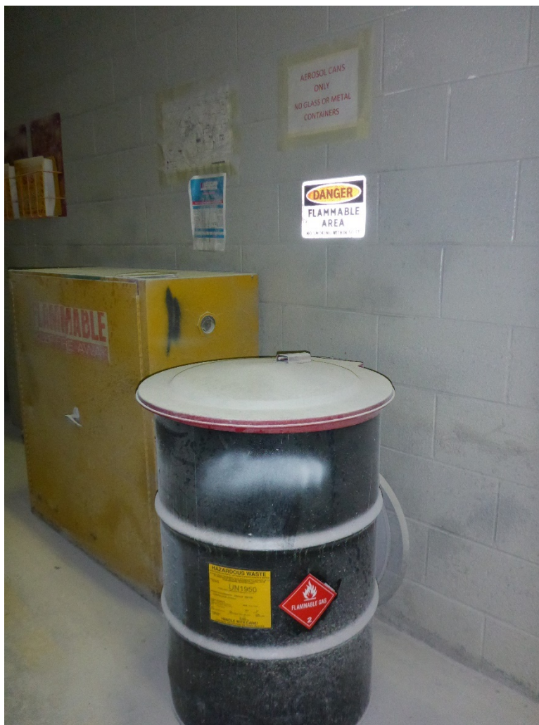
Photo 12: SAA for accumulating waste aerosol cans in the Metal Plant. 55-gallon drum with flip-top lid labeled D001 / F003 / F005 hazardous waste aerosols.
