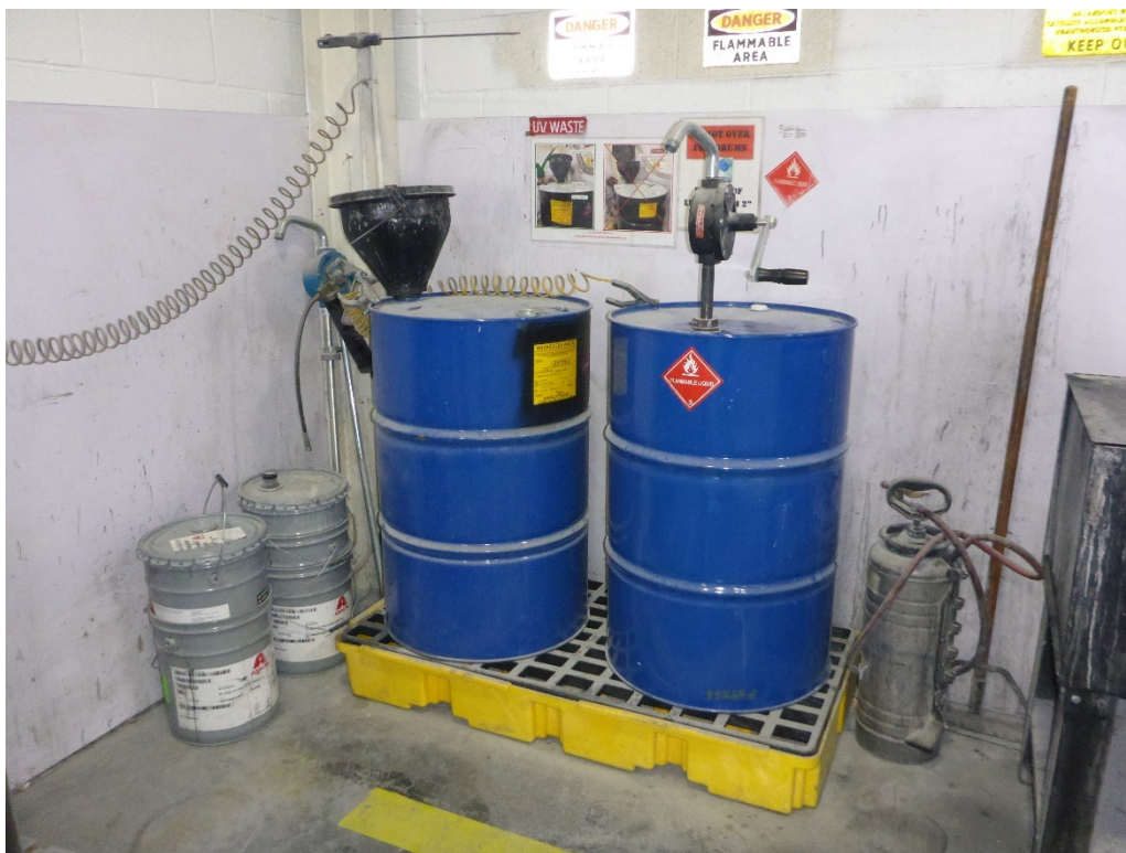
Photo 17: Resin Plant SAA for accumulating contaminated spent solvent generated during cleanup activities in the UV area. 55-gallon drum with flip-top funnel lid labeled D001 / F003 hazardous waste recycled solvent.
