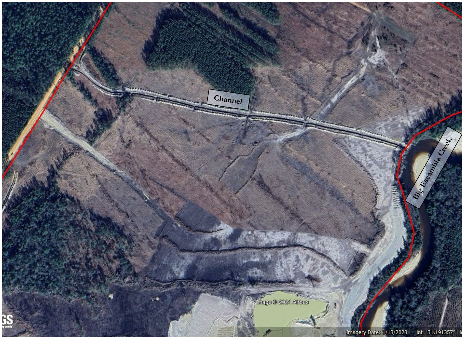
Figure 4. GoogleEarth aerial image of an excavated channel leading across the northern area of the Facility, imagery dated January 13, 2023. The channel flow path leads from west to east and to Big Escambia Creek. The red lines indicate the approximate Facility boundary.
