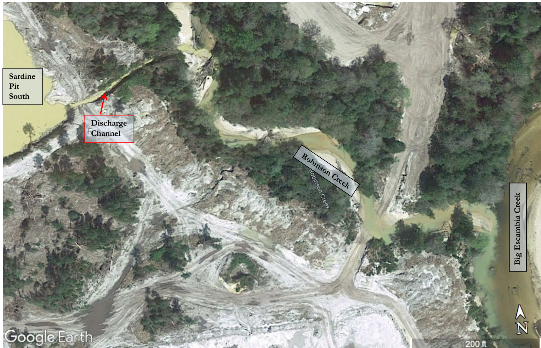
Figure 6. GoogleEarth aerial image of the Sardine Pit South and a surface water discharge channel leading from the Pit to Robinson Creek and ultimately to Big Escambia Creek. Approximate imagery date 2016. Note the change in water clarity of both Robinson Creek and Big Escambia Creek upstream and downstream of the discharge channel.
