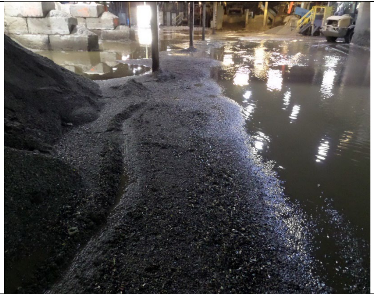
Keebler Plant Building Filter Cake Pile. The inspectors observed wastewater and solids accumulating on the concrete floor next to the Pile. Photograph 46 taken at 2:38 p.m.
