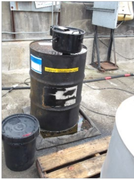
Picture 19: Labeled used oil collection drum
