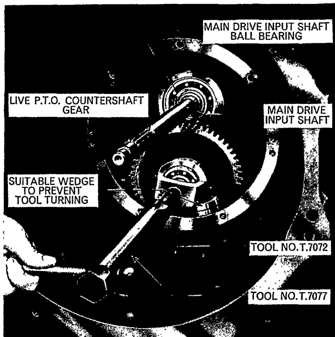
Figure 14(A) Removing Live P.T.O. Countershaft Front Bearing
