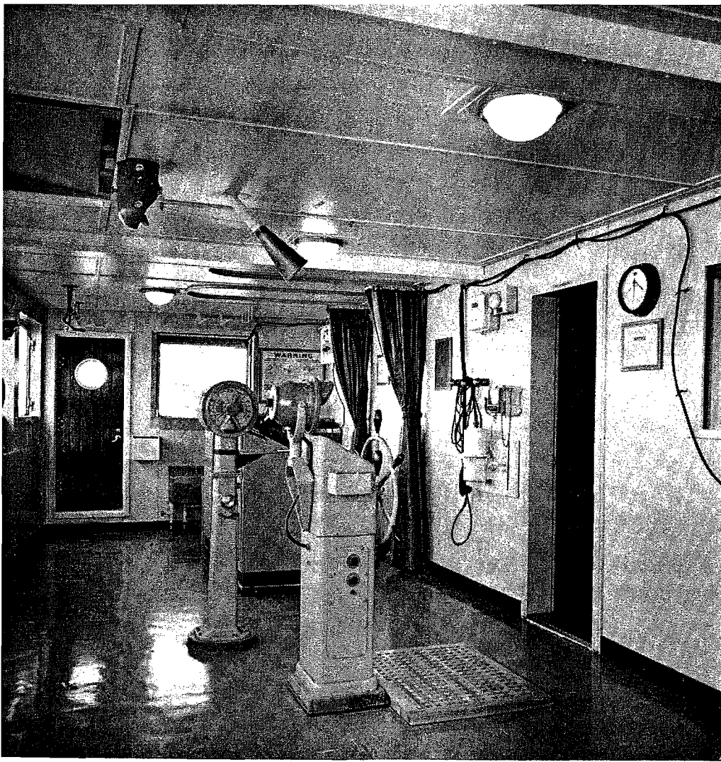
Partial view of the navigation bridge on the ESSO BOSTON. Radar viewing screens can be seen behind the engine room telegraph.
