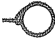
Bad—Because of cutting action running line can of eye splice can break loose.
