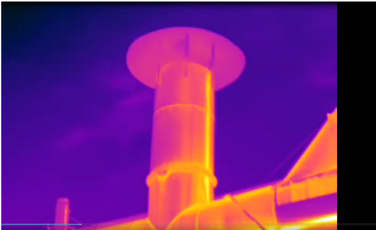
Photo 2: Main Bypass Stack Demonstrating Leaks on Camera's Auto Mode
