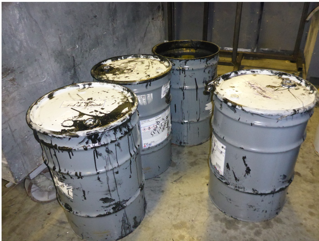
Photo 9: Four 30-gallon drums of hazardous waste DAA / IMC mixture staged for scraping and consolidation. One drum had no lid. None of the drums were labeled or marked with an indication of the hazards of the contents.
