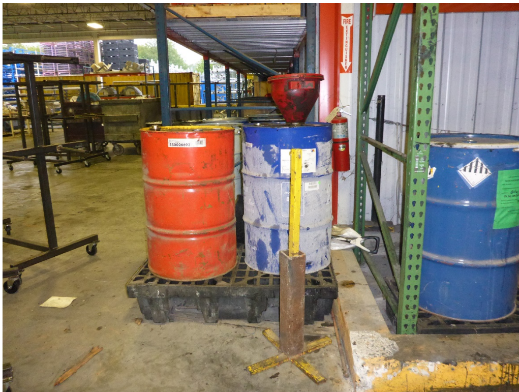
Photo 8: 55-gallon drum to accumulate used oil. Drum equipped with a latched funnel in the lid, but it was not labeled as “used oil.”
