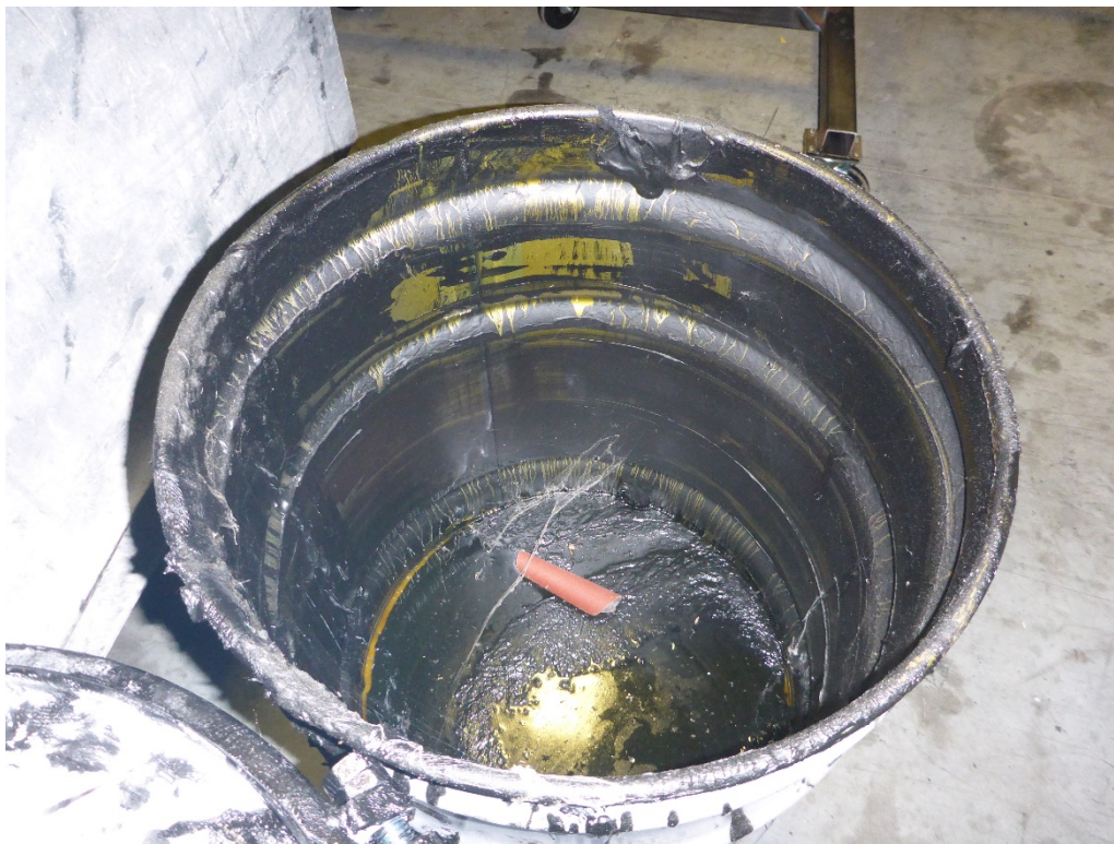
Photo 10: One of four 30-gallon drums of hazardous waste DAA / IMC mixture staged for scraping and consolidation. Drum has no lid and is approximately 1/3 full. Drum was not labeled or marked with an indication of the hazards of the contents.
