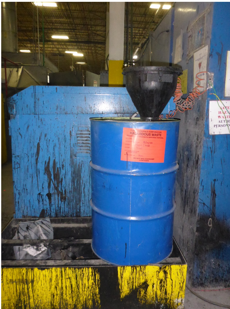
Photo 1: One 55-gallon drum located in the SAA next to the paint booth for accumulating D001 hazardous waste paint solvent and MAK. This drum was not marked with an indication of the hazards of its contents.
