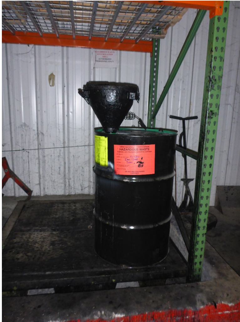
Photo 5: 55-gallon hazardous waste storage drum accumulating and storing hazardous waste IMC / DAA generated at the press lines. Drum observed in the CAA located in the covered area just outside of and adjacent to the manufacturing building. Drum was not marked with an indication of the hazards of its contents.
