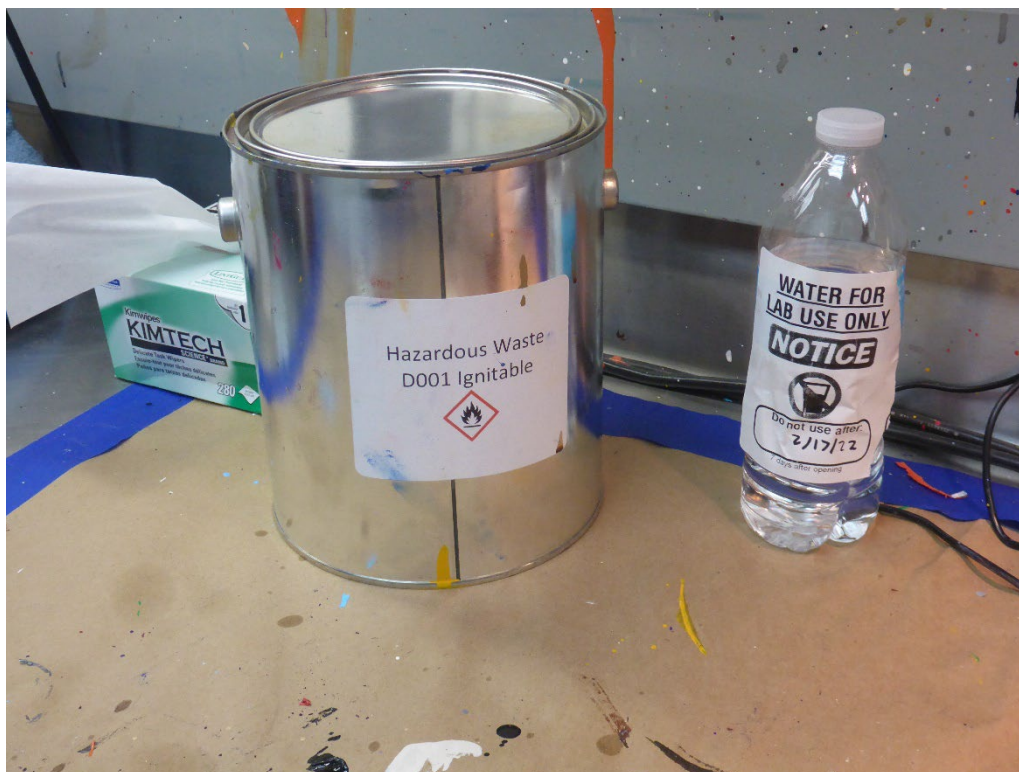
Photo 14: One 1-gallon paint can, which was observed in the Laboratory SAA for managing hazardous waste flammable liquids. The container was labeled D001 hazardous waste flammable liquid and marked with a flammable pictogram.
