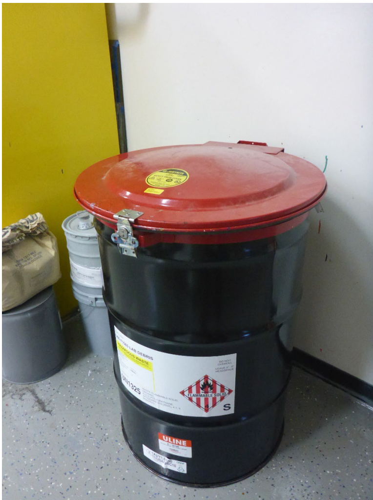
Photo 12: One 55-gallon drum observed in the Laboratory SAA for managing hazardous waste lab debris. The drum was identified as U80-11585 lab debris, labeled D001 hazardous waste flammable solid (polyurethane Stoddard solvent), and marked with a flammable solid DOT hazard placard.
