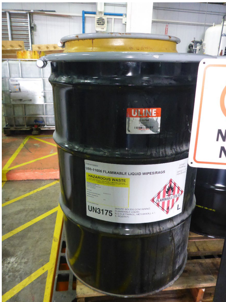
Photo 31: One 55-gallon drum labeled hazardous waste flammable liquid cups / rags (ethanol / methanol) and identified with a flammable solid DOT hazard placard. The drum was not marked with an accumulation start date.
