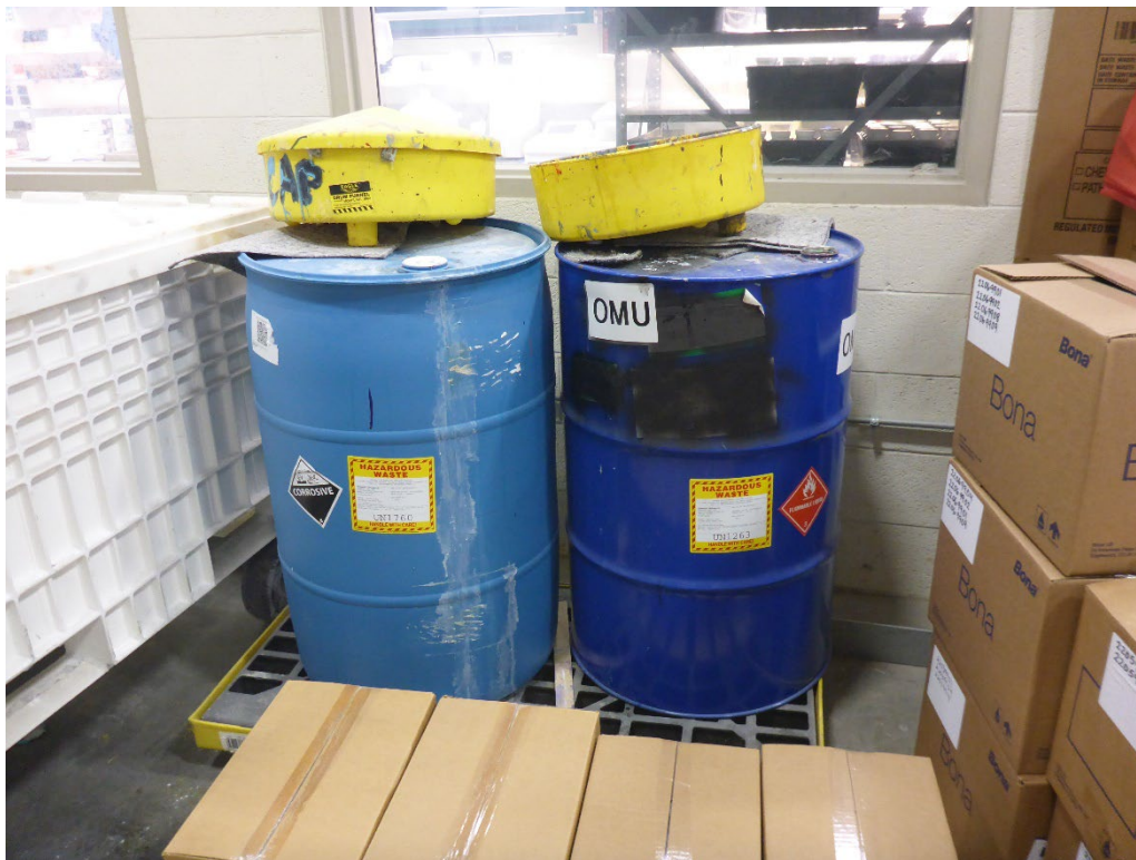
Photo 16: One 55-gallon steel drum, which was observed in the Laboratory SAA for managing hazardous waste paint waste. The container was labeled D001 hazardous waste paint waste (polyurethane / Stoddard solvent) and marked with a flammable liquid DOT hazard placard. One 55-gallon poly drum, which was observed in the Laboratory SAA for managing hazardous waste titration waste. The container was labeled D002 hazardous waste titration waste (sulfuric acid / hydrogen peroxide) and identified with a corrosive DOT hazard placard.
