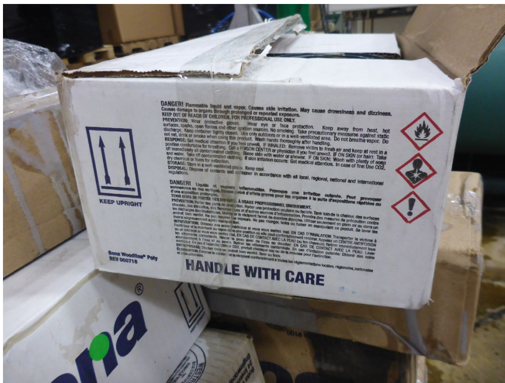
Photo 20: Smaller containers ready for consolidation in the cubic yard box in the Main CAA. Containers are identified with the color-coding dot, but they are not labeled as hazardous waste, marked with an accumulation start date, or identified with an indication of the hazards of their contents. Some smaller containers are also open or in poor condition.
