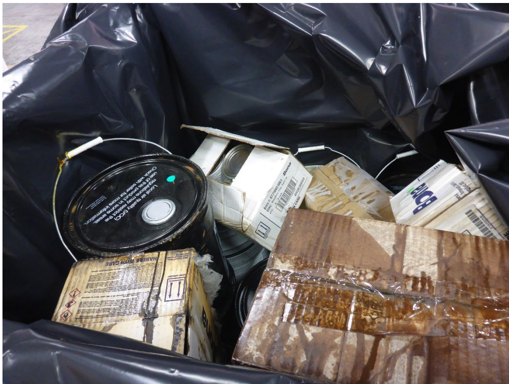
Photo 21: Smaller containers that have been consolidated into a cubic yard box in the Main CAA. The cubic yard box is open, not labeled as hazardous waste, not marked with an accumulation start date, and not identified with an indication of the hazards of its contents.
