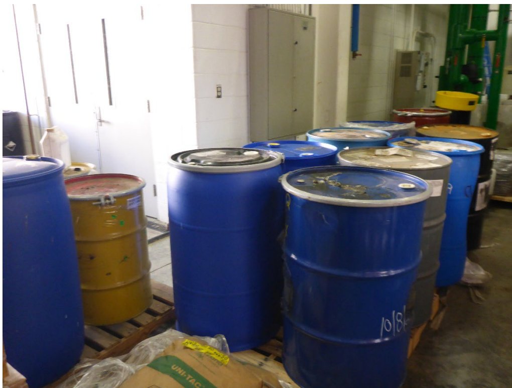
Photo 23: Approximately twenty 55-gallon drums staged in the area designated for waste-pickup. None of the containers were labeled as hazardous waste, and many were not marked with an accumulation start date or identified with an indication of the hazards of their contents.
