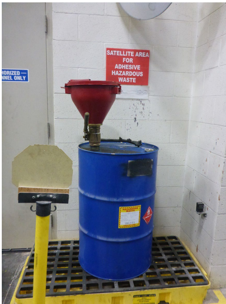
Photo 15: One 55-gallon drum, which was observed in the Laboratory SAA for managing hazardous waste excess cleaning solvents. The container was labeled D001 hazardous waste adhesive solvent titrant (ethanol / methanol) and marked with a flammable liquid DOT hazard placard.
