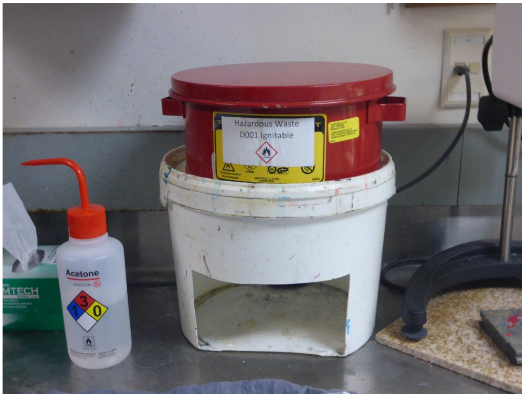
Photo 13: One ½-gallon flammable can, which was observed in the Laboratory SAA for managing hazardous waste flammable liquids. The container was labeled D001 hazardous waste flammable liquid and marked with a flammable pictogram.
