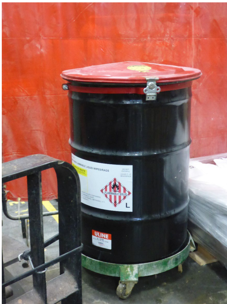
Photo 36: One 55-gallon drum observed in the Adhesives Area SAA for managing hazardous waste flammable solids. The drum was labeled D001 hazardous waste flammable liquid cups / rags (ethanol / methanol) and marked with a flammable solid DOT hazard placard.
