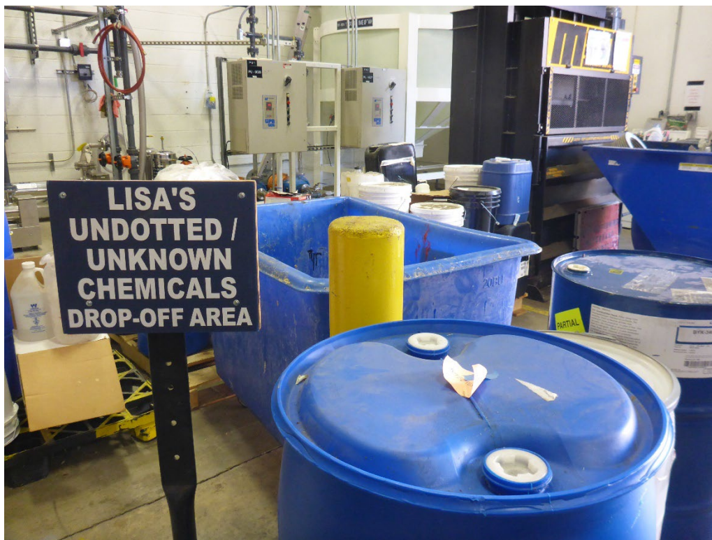
Photo 25: Area for staging wastes that are transferred to the Main CAA from SAAs or staging unknown materials that are included with customer returns.
