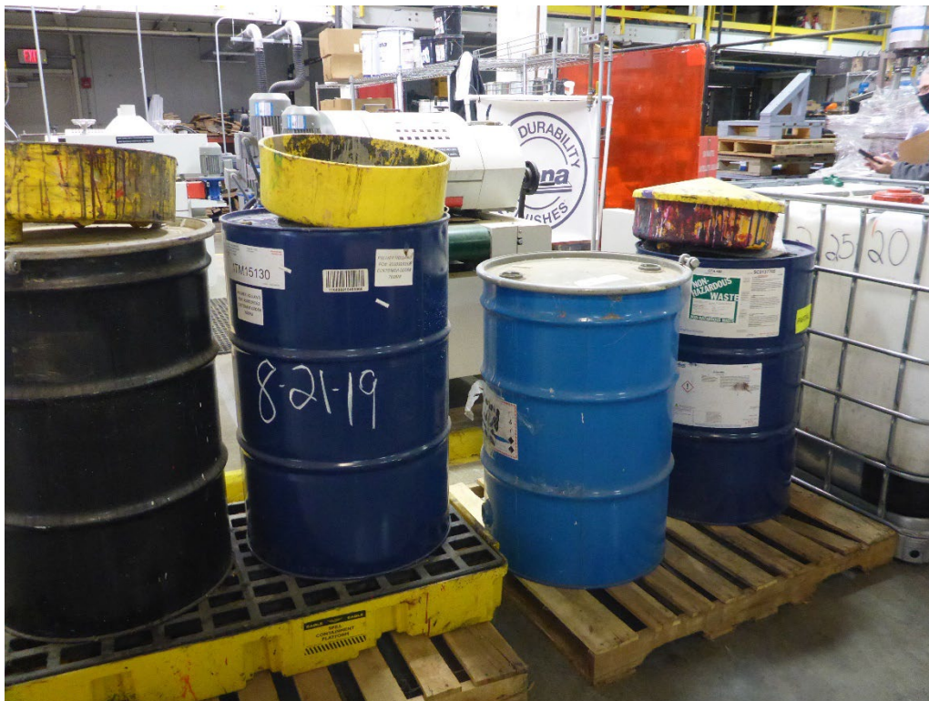
Photo 32: Four 55-gallon drums used to accumulate wastes generated in the UV Area.
