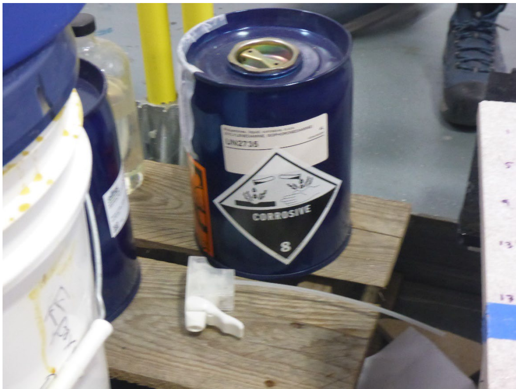
Photo 7: One of two 1-gallon blue containers of corrosive material which were among the miscellaneous materials observed in an area next to a metal handrail outside of the Laboratory in the Filling Area.
