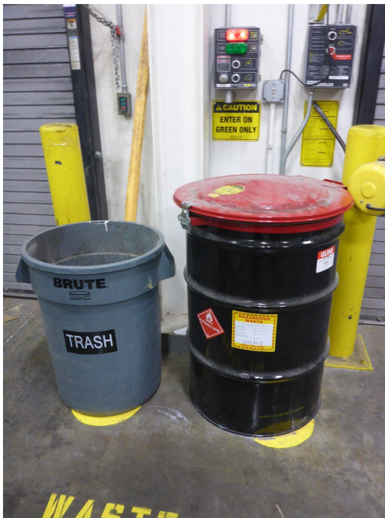
Photo 18: One 55-gallon drum, which was observed in the Shipping and Receiving SAA for managing hazardous waste aerosol cans. The container was labeled D001 / D005 / D035 hazardous waste aerosols and marked with a flammable liquid DOT hazard placard. The container was not marked with an indication that the contents are toxic.
