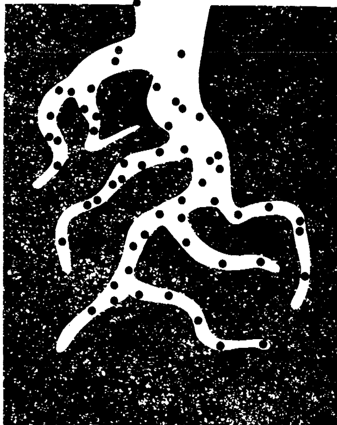
Figure 1a — Concept of molecules in activated charcoal pores
