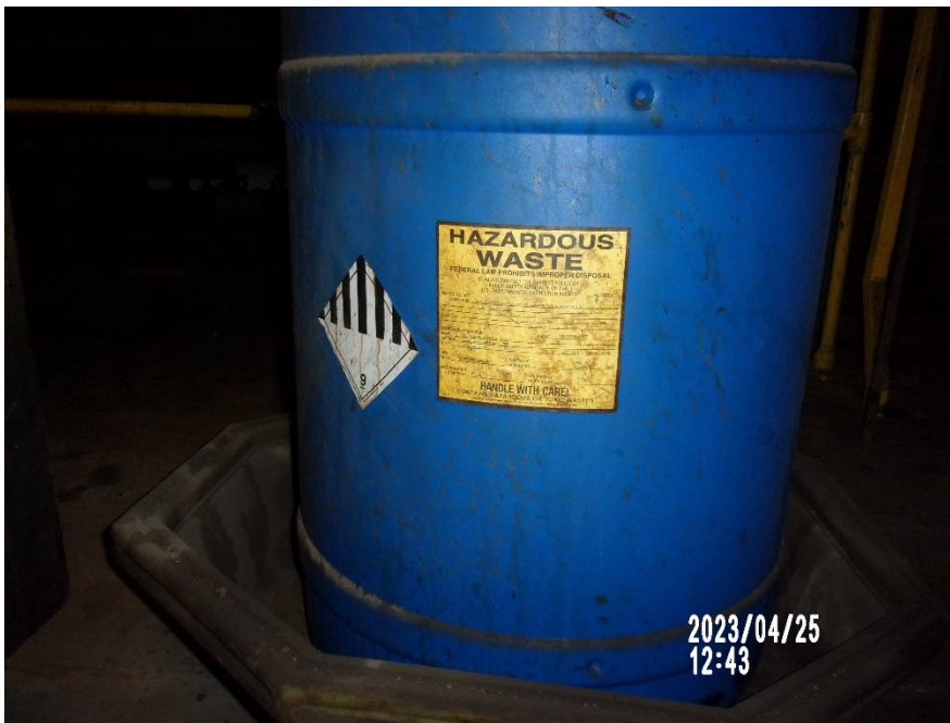
Photograph 9 – Hazardous Waste Label and Class 9 DOT Label
