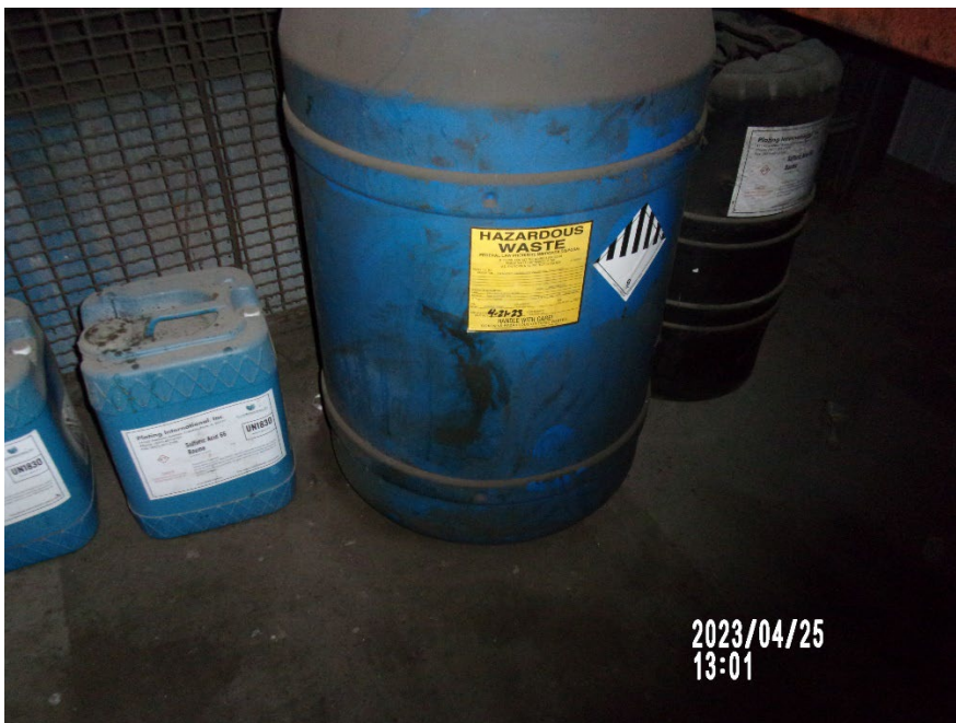
Photograph 10 – 90-Day CAA Hazardous Waste Drum With Class 9 DOT Label
