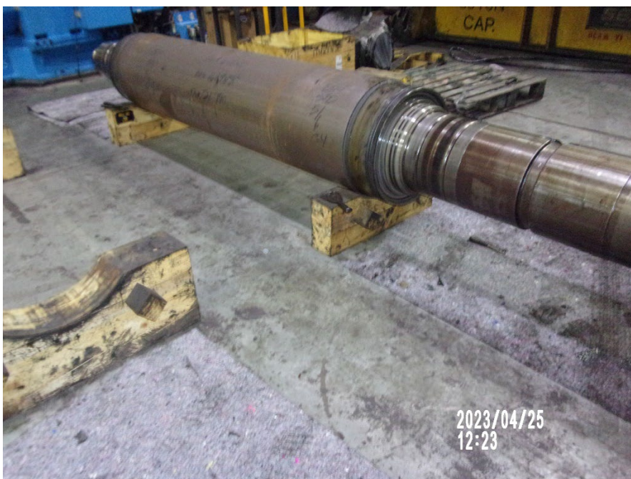
Photograph 4 – Used Steel Mill Roll from SDC in Roll Shop
