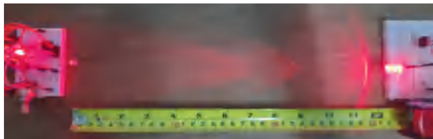
Fig. 25.8 Data transmission of LiFi system in certain distance
