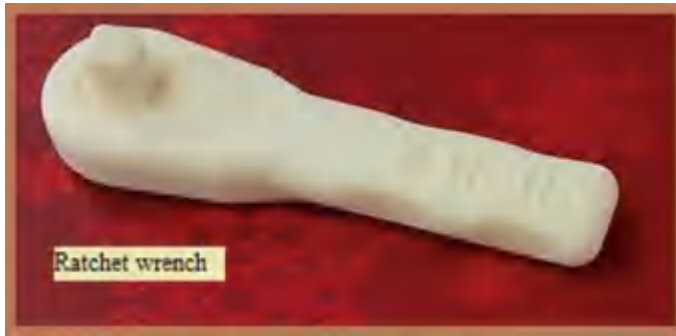
Fig. 9.12 3D printed ratchet wrench
