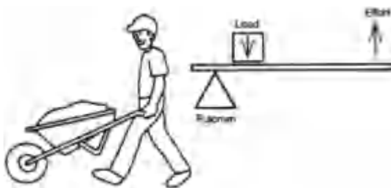
Fig. 30.1 Wheelbarrow applying second class lever
