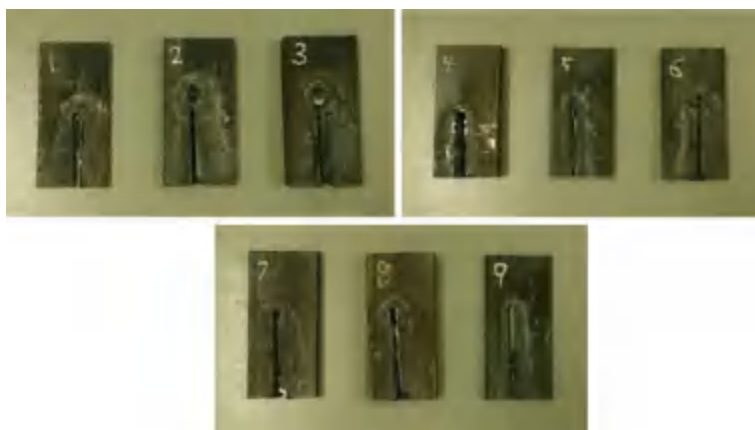
Fig. 21.3 Specimens fabricated based on L9 Taguchi method
