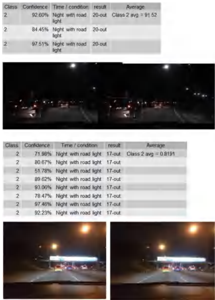
Fig. 4.10 Vehicle detection during the night with road lights
