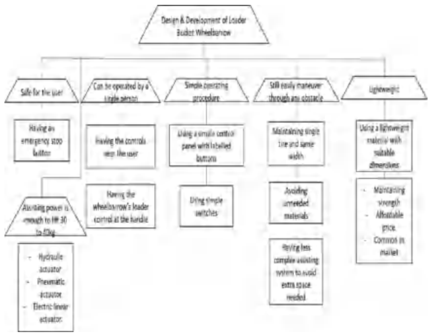
Fig. 30.3 Objective tree of wheelbarrow loader bucket design
