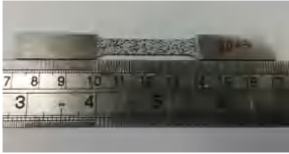
Fig. 10.1 Tensile specimen with matte black and white uniformly distributed speckles
