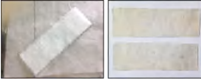
Fig. 1.2 Skin composites of fiberglass
