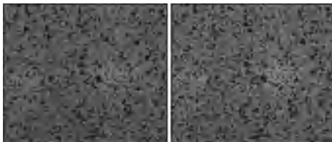
Fig. 24.2 Views from each cameras which should be focussed on the same location on the sample, preferably at the centre. (Left) view from camera 1 and (Right) view from camera 2. Together, the two images will be processed to enable stereo vision
