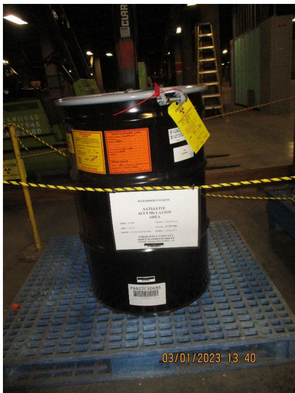
Photograph 49: 55-gallon Hazardous Waste Drum in SAA S-337-06.
