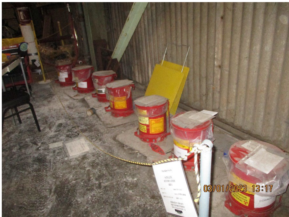
Photograph 44: 5-gallon hazardous waste containers in SAA S-335-Central.
