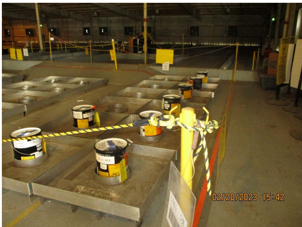
Photograph 20: Hazardous waste fissile material containers separated by metal pallet spacing.
