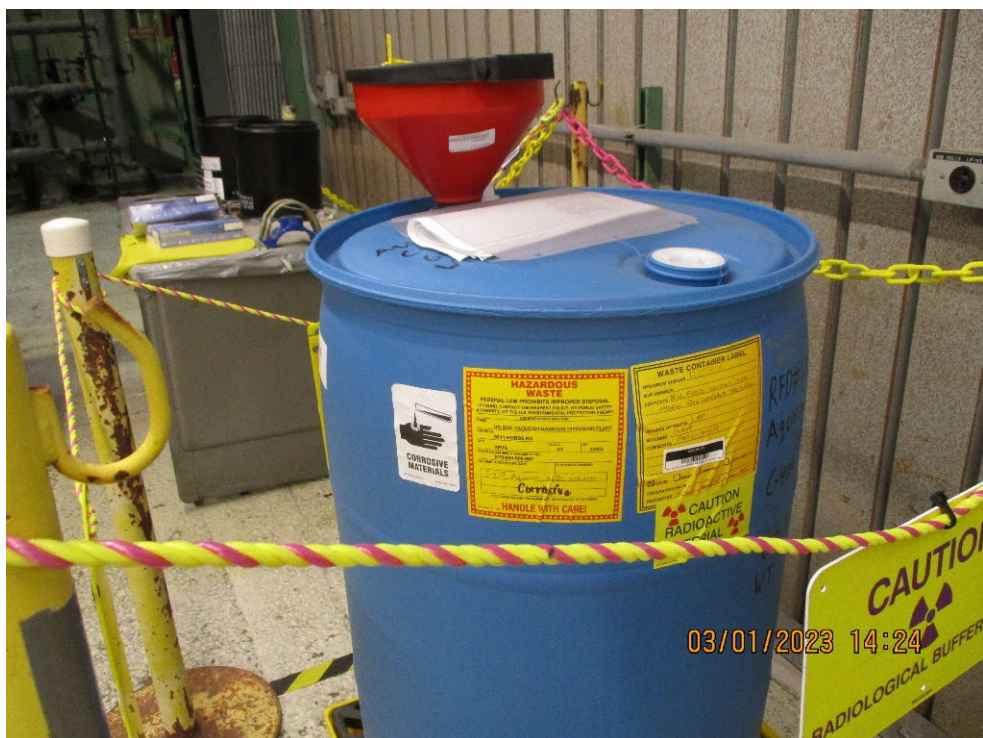
Photograph 64: 55-gallon Satellite Container with Corrosive, Non-Fissile, Aqueous Waste.
