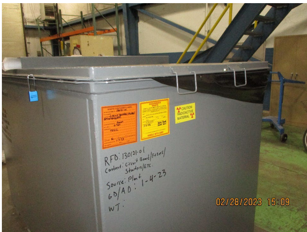
Photograph 15: ST-90 Hazardous Waste Storage Container.
