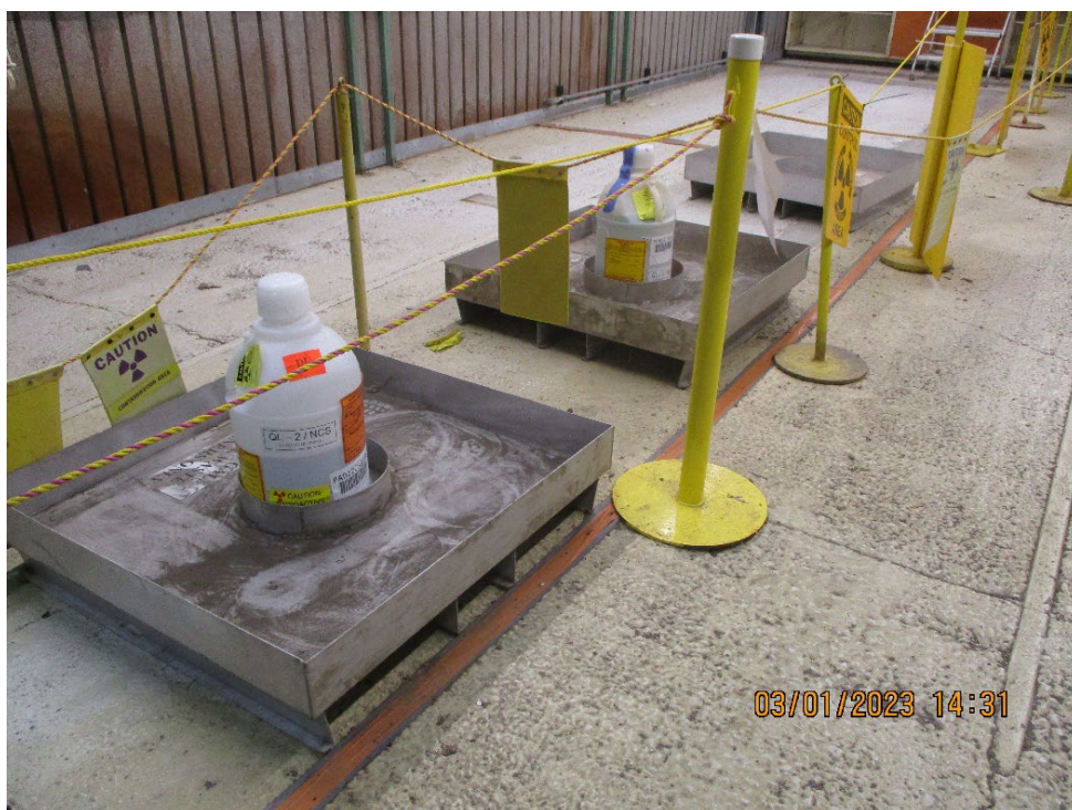
Photograph 65: Satellite Containers with fissile material.
