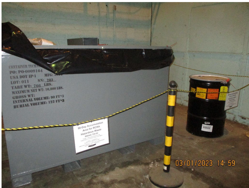
Photograph 71: ST-90 and 55-Gallon Hazardous Waste Containers in 90DAA-720-02.
