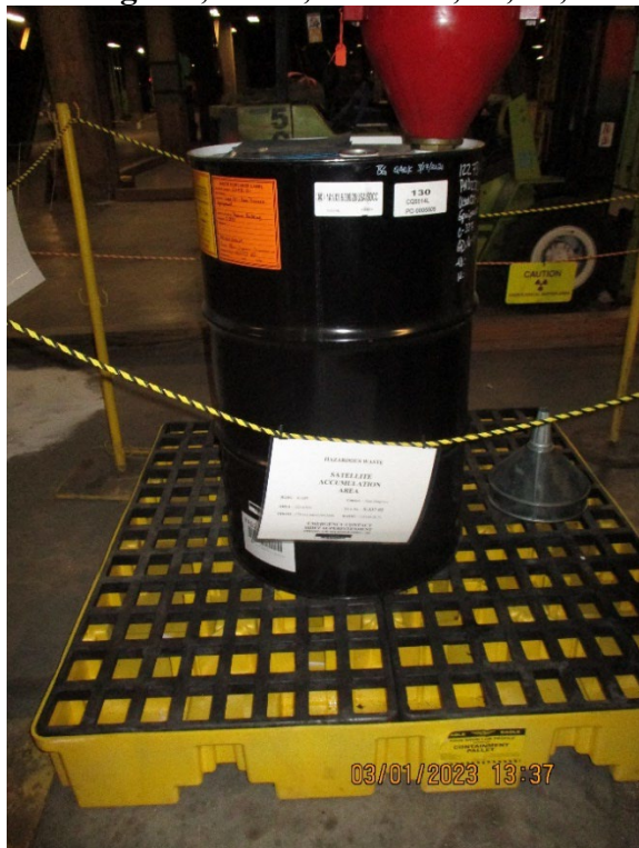
Photograph 47: 55-gallon Hazardous Waste Drum in SAA S-337-02
