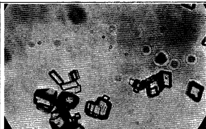
Pure \text{CaCO}_3 , 450 magnifications.
