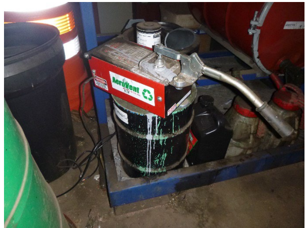
Photograph 16: Aerosol SAA Container with puncture Device.
