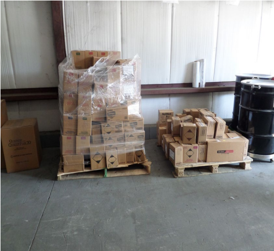
Formulated Solutions, LLC (Formulated). 90-Day or Less Accumulation Area. Observed five pallets each accumulating several boxes of spent aerosols. Observed the boxes were not marked or labeled with the words universal waste. Photograph 1 taken at 10:55 a.m.
