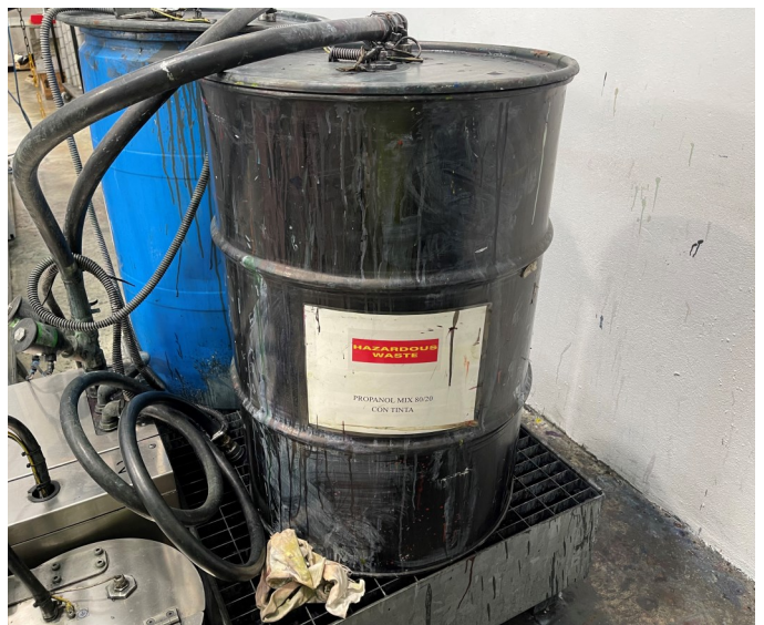
Picture 4 - ALCO HIGH TECH PLASTICS - At the Plastic Extrusion area (SOMA), there was a second SSA with one (1) 55 -gallon black drum with with spent liquid solvent waste containing a mixture of propanol and ink, labeled as “Hazardous Waste,” and not identified with its hazard communication pictogram as “Flammable Liquids.”
