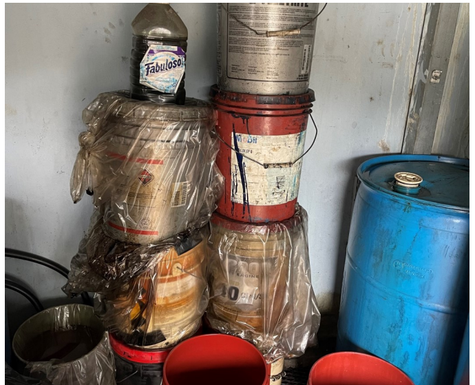
Picture 20 - ALCO HIGH TECH PLASTICS- At the Oil Storage area, I observed seven (7) 5-gallon orange/gray plastic containers with used oil not marked with the words, "Used Oil"
