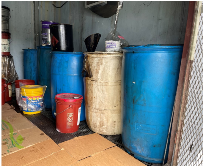
Picture 19-ALCO HIGH TECH PLASTICS- At the Used Oil Storage area, I observed five (5) 55-gallon blue/white plastic drums with used oil not marked with the words, "Used Oil."
