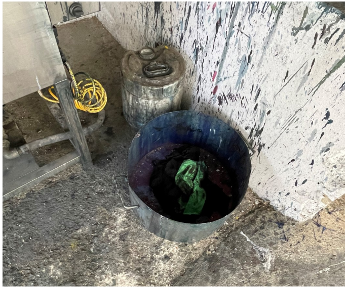
Picture 9 - ALCO HIGH TECH PLASTICS - At the Alcohol Warehouse, I observed one (1) ½-cut 55-gallon blue plastic drum “open” with impacted rags contaminated with spent liquid solvent waste of a mixture of propanol and ink, not labeled as “Hazardous Waste,” nor identified with its hazard communication pictogram as “Flammable Solids.”
