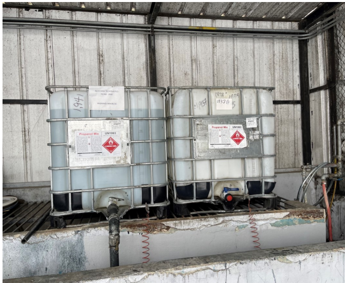
Picture 7 - ALCO HIGH TECH PLASTICS - At the the Alcohol Warehouse area, it was observed that all Propanol Mix 80/20 solvent products (i.e., UN 1993 – Flammable Liquids) are stored in two (2) 275-gallon totes for future use in plastic printing machines.
