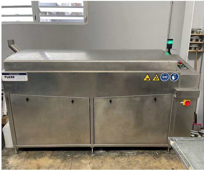
Picture 5 - ALCO HIGH TECH PLASTICS - At the Plastic Extrusion area (SOMA), there was a third SSA with one (1) 300-gallon stainless steel tank used to clean anilox rollers not labeled with the words, “Hazardous Waste,” nor identified with its hazard communication pictogram as “Corrosive Liquids.”
