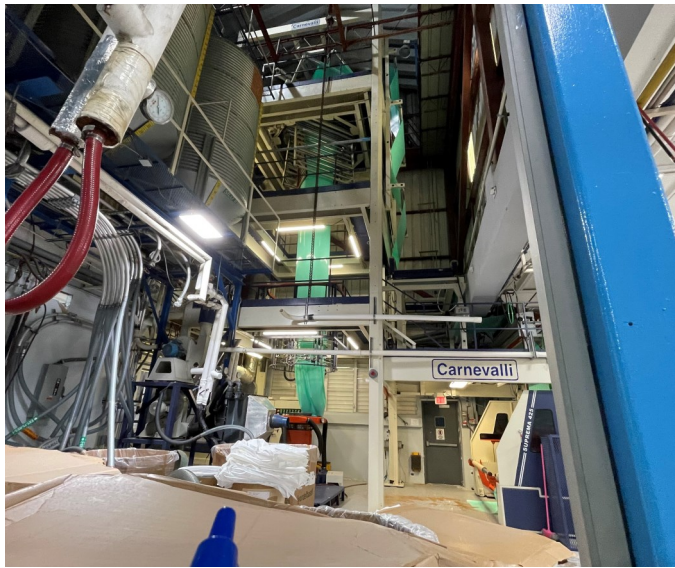
Picture 1 - ALCO HIGH TECH PLASTICS - At the Plastic Extrusion area, a high-volume manufacturing process is undertaken where raw plastic (pellets) is melted and formed into a continuous plastic layer.
