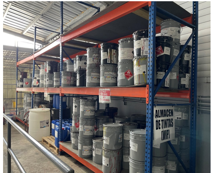
Picture 6 - ALCO HIGH TECH PLASTICS - At the Ink Warehouse area EPA Inspector observed that all new ink products are stored in 5-gallon pails (i.e., Cyan, Magenta, Yellow and Black) for immediate use in plastic printing machines.
