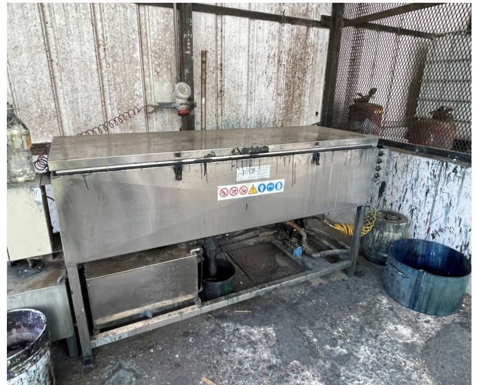
Picture 8 - ALCO HIGH TECH PLASTICS — At the Alcohol Warehouse, I observed a part-washer machine that was used to clean anilox and/or plaster rollers until the new SAA Washing Machine unit was installed nearby the plastic printing machines. This part-washer has been discontinued and emptied over a year ago and is not currently in use.
