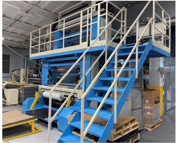
Picture 2 - ALCO HIGH TECH PLASTICS - At the Plastic Extrusion area, the material is gradually melted by the mechanical energy generated by turning screws and by heaters arranged along the barrel of the extruder.
