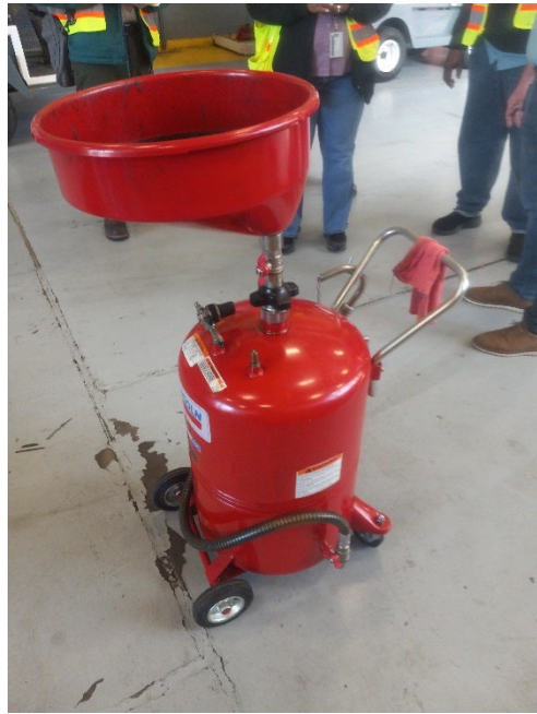
Photograph 62 – 5400 NTVB rolling used oil storage
