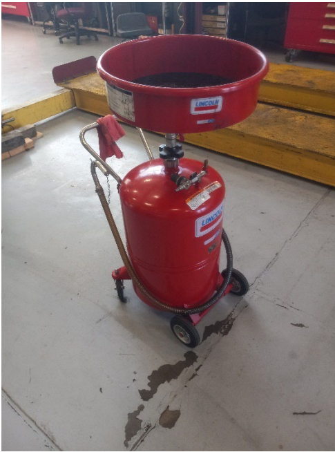
Photograph 61 – 5400 NTVB rolling used oil storage
