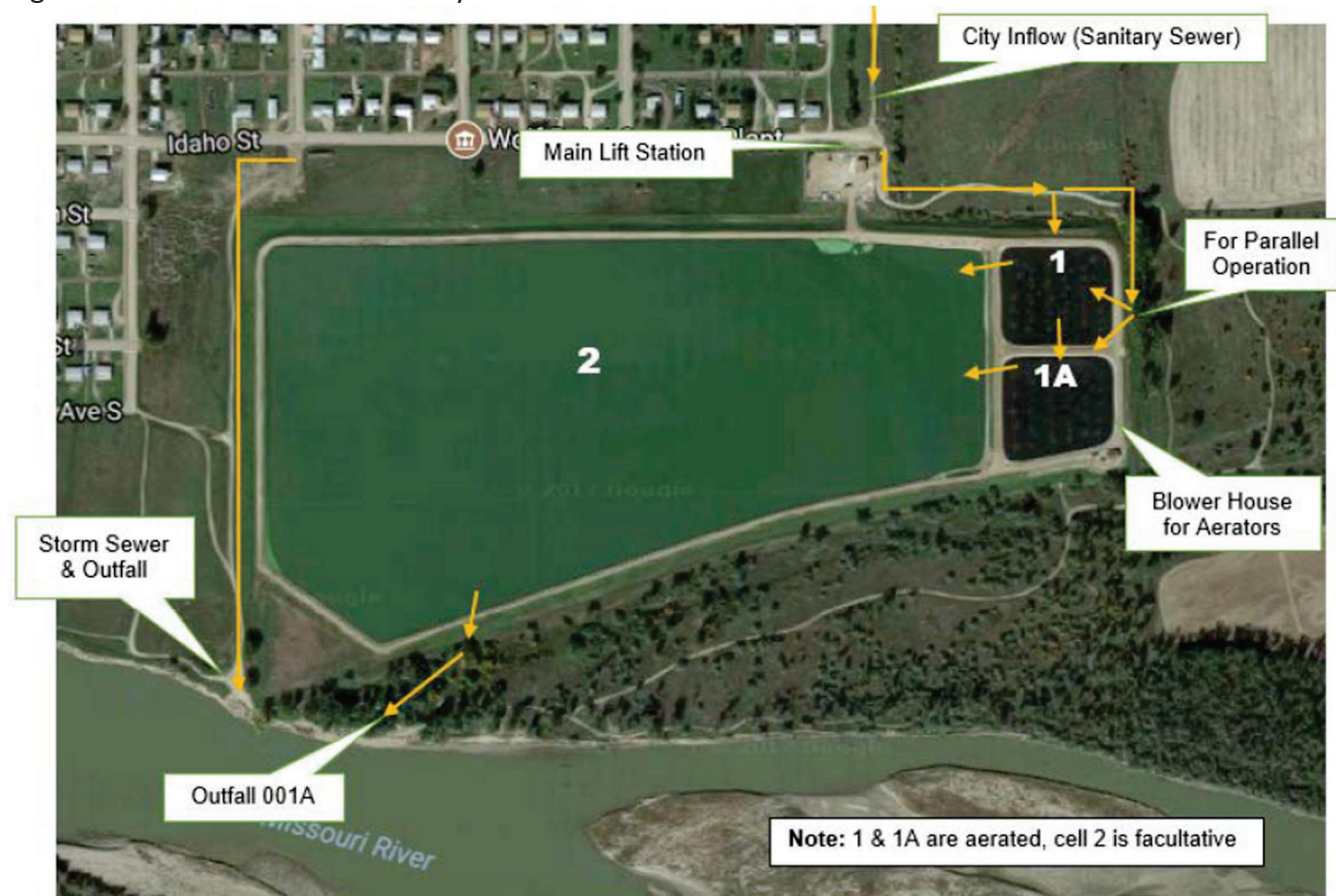
Figure 1: Wastewater Treatment System
