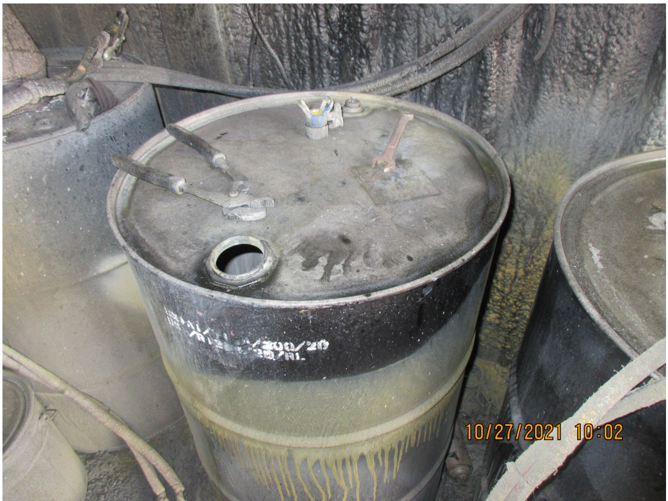
Photo 5 – Top of one of four drums containing spent acetone in SAA
