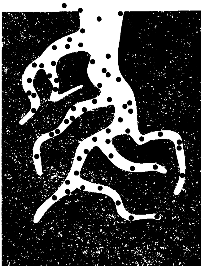
Figure 1a — Concept of molecules in activated charcoal pores
