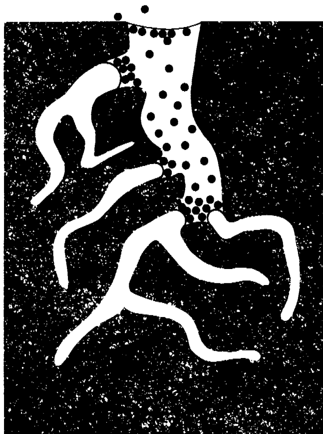
Figure 1b — Menisci formation by molecules in activated charcoal pores
