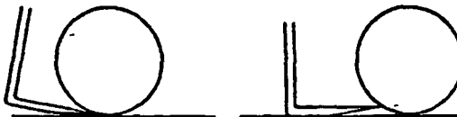
FIG 22-12 - To pick up round objects, forks should be tilted (left), not used flat (right)
