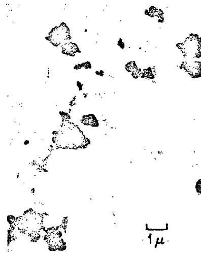
Figure 3. Decomposition product from normal wear of brake lining.
