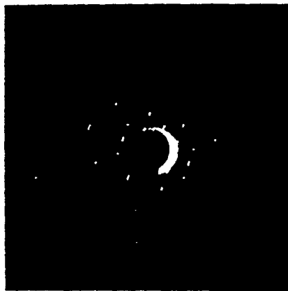
Fig. 2. Selected area electron diffraction pattern (SAED) of a chrysotile asbestos fibril
