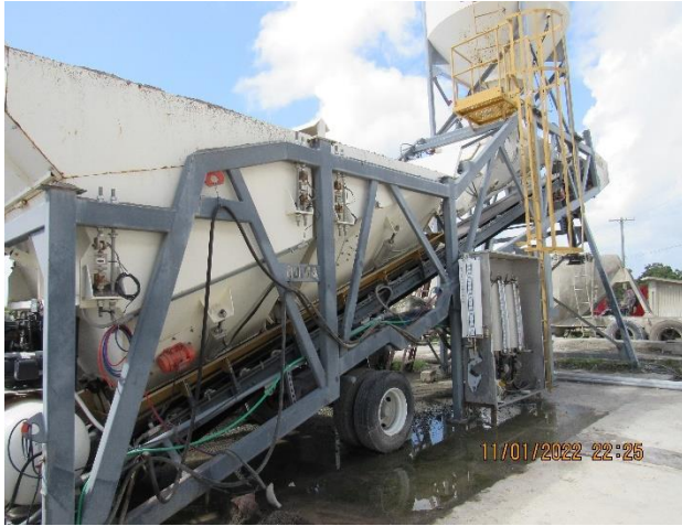
IMG 785 -Accumulation of water beneath ready-mix concrete batch plant related to operations of the system. Source of a dry-weather flow observed.
