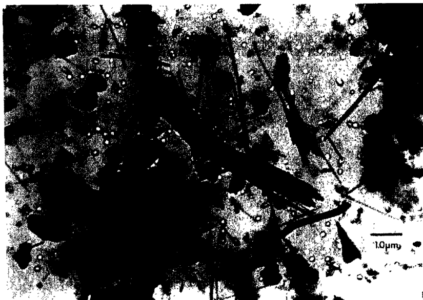
FIGURE 3. Material collected from the surface of the used clutches contained various types of chrysotile structures. Magnification 12,000×
