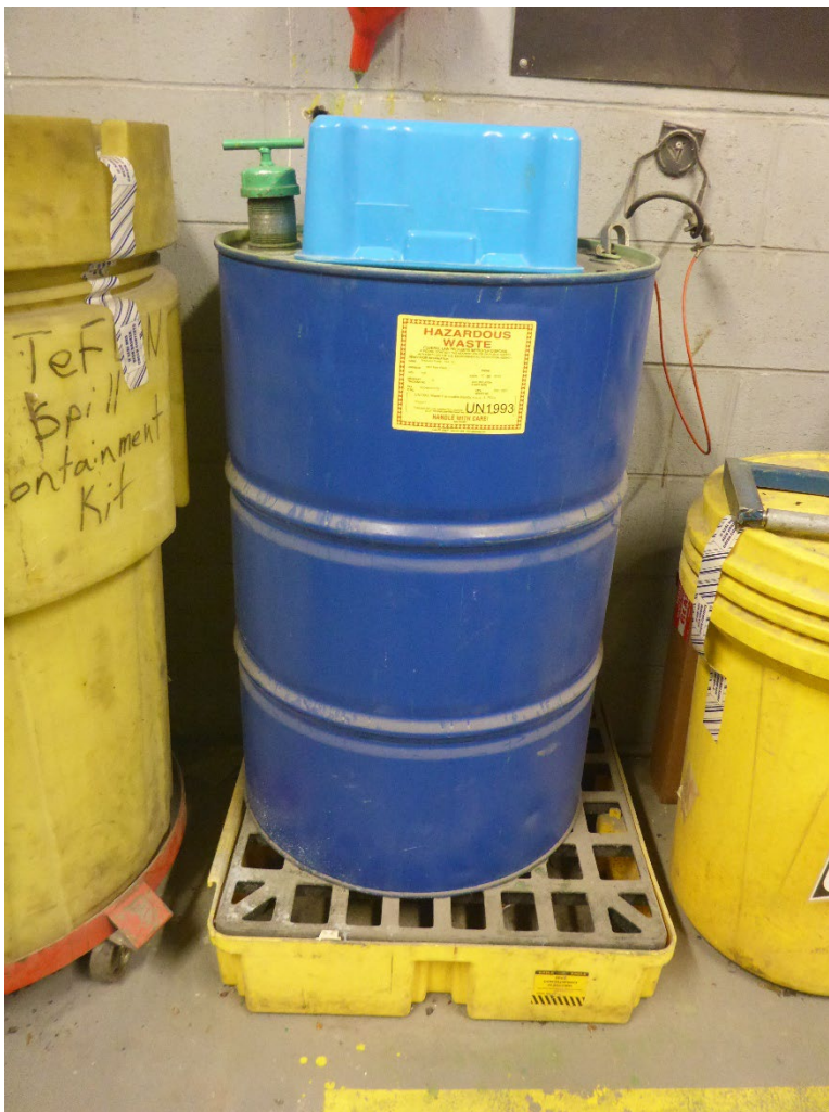
Photo 14: One 55-gallon drum of D001 / D007 hazardous waste flammable liquids in one of two SAAs inside the Teflon Room. The drum is labeled hazardous waste and identified as a flammable liquid, but it is not marked with an indication that the contents are toxic.
