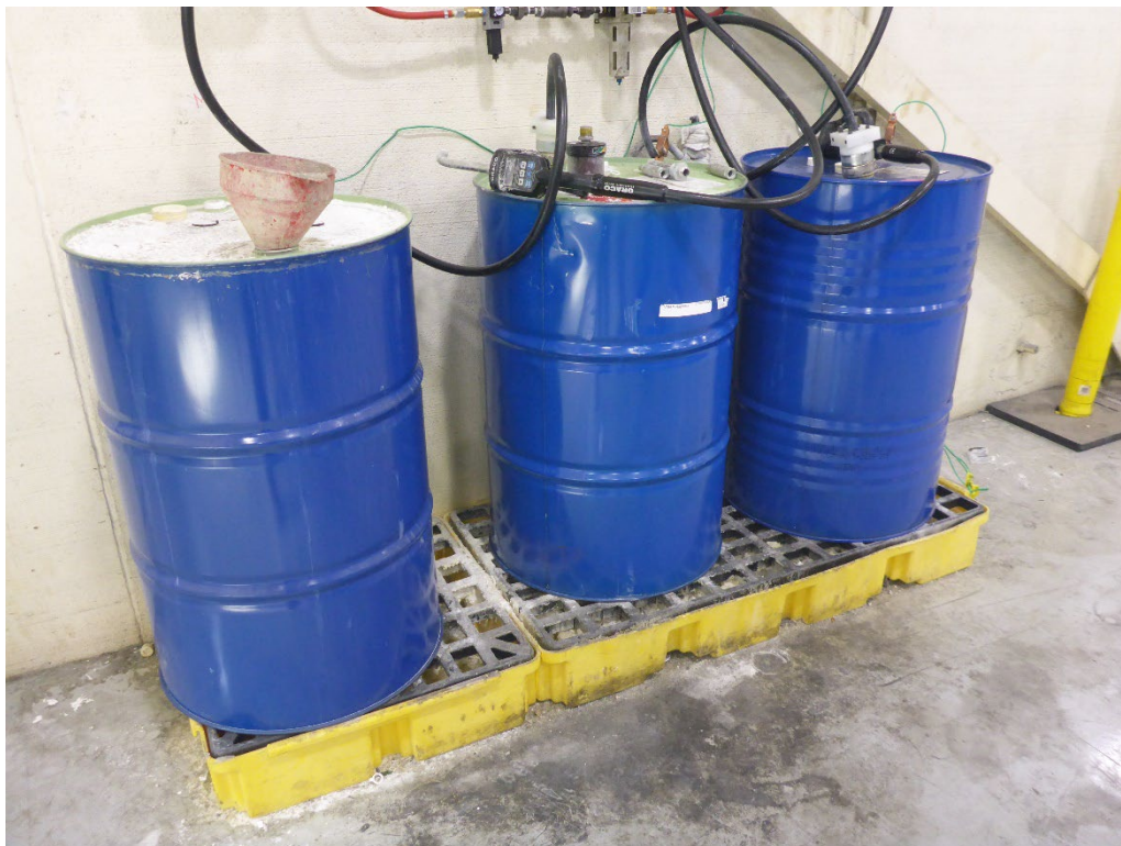
Photo 1: Three 55-gallon drums on portable secondary containment pallets at the Fiber One Single Spin Machine Area SAA. The drum on the left, which contains hazardous waste naphtha primer liquid mixture, was not closed or labeled.
