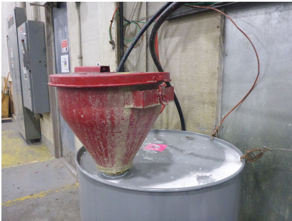
Photo 12: Unlatched funnel on the drum of hazardous waste isopropanol in the Molded Area Primer Station SAA.
