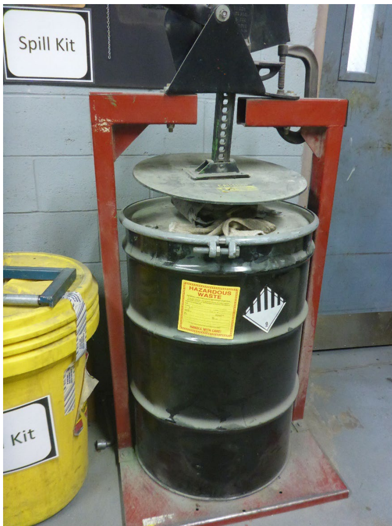
Photo 15: One 55-gallon drum of D007 hazardous waste solids in one of two SAAs inside the Teflon Room. The drum is labeled hazardous waste and identified with a DOT class 9 hazard placard, but it is not marked with an indication that the contents are toxic.
