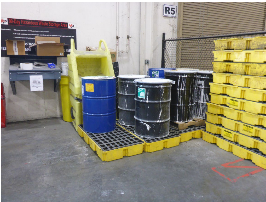
Photo 6: Eight 55-gallon drums located in the far corner immediately to the left inside the entrance to the caged CAA. The drum on the left contains D001 hazardous waste flammable liquids (naphtha, propyl acetate), and the remaining seven drums contain nonhazardous waste.
