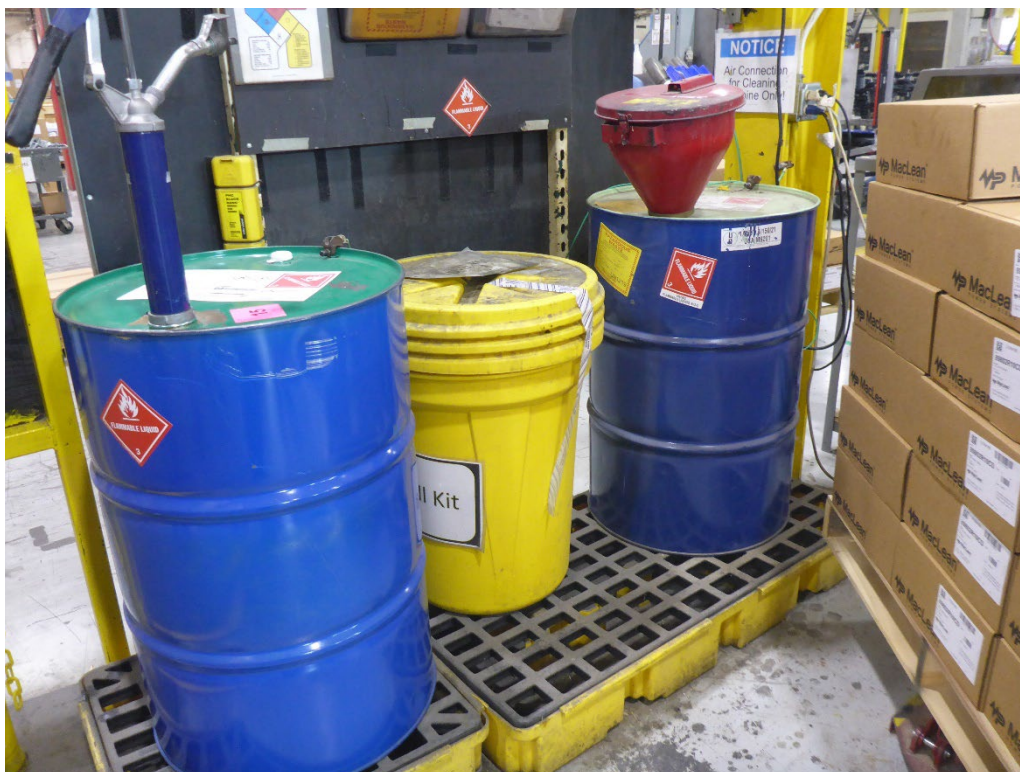
Photo 4: Two 55-gallon drums and a spill kit at the Cut Out Area SAA. The drum on the right contains D001 hazardous waste isopropanol.
