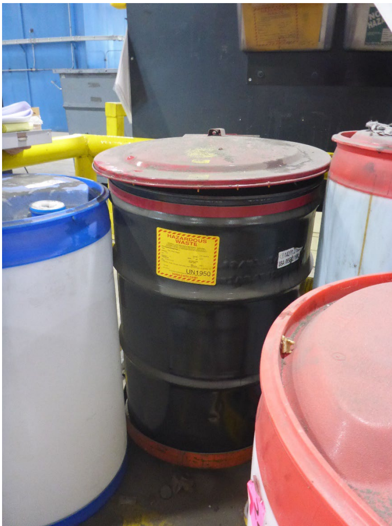
Photo 13: One 55-gallon drum of D001 hazardous waste aerosols in the SmartFoam Part A & B SAA. The lid did not make complete contact between the lid and the rim of the drum.
