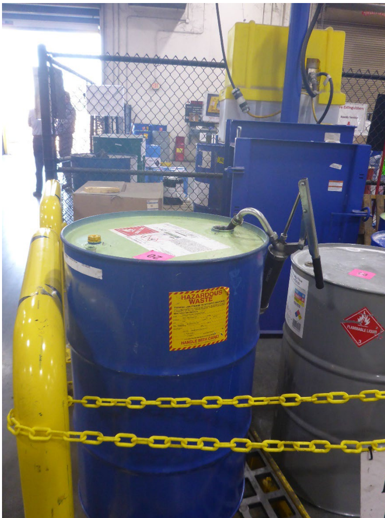
Photo 8: One 55-gallon drum of hazardous waste isopropanol in the SAA located outside of the caged CAA. The bung had been removed from the drum, leaving the container open.
