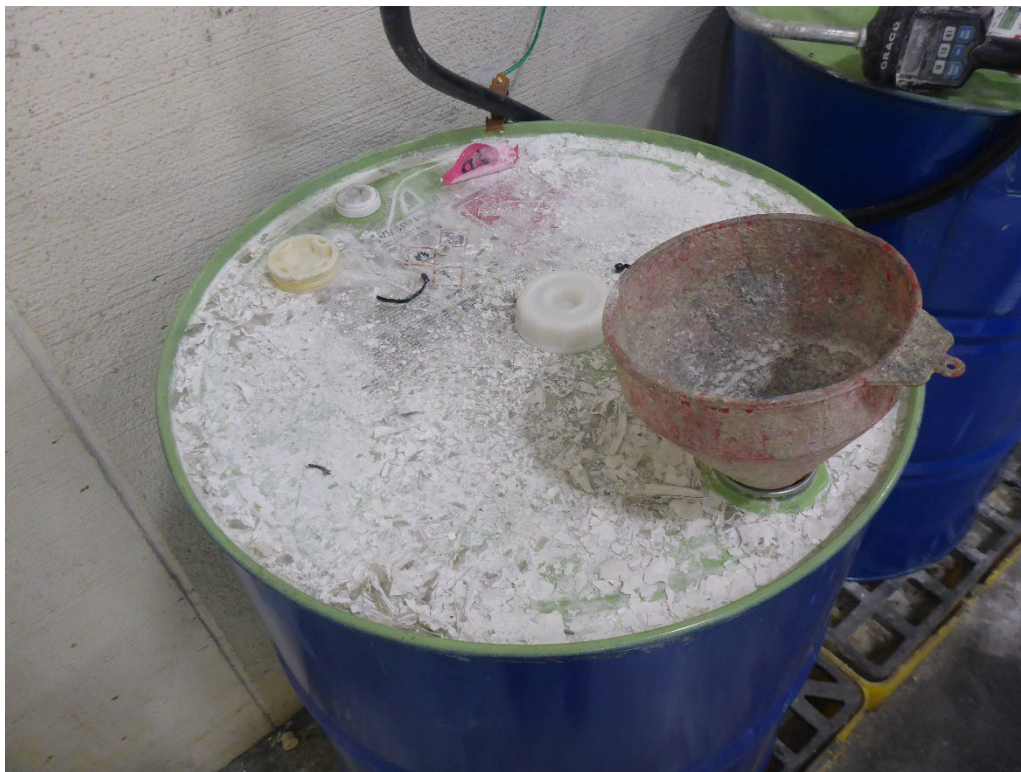
Photo 2: Open funnel in the container of hazardous waste naphtha primer liquid mixture at the Fiber One Single Spin Machine Area SAA.
