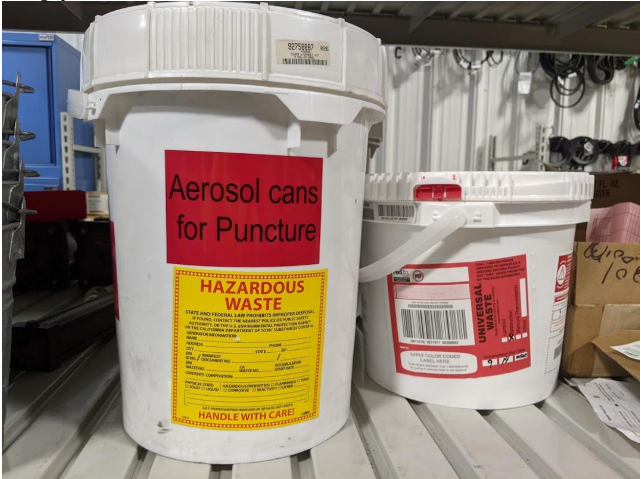
Photograph 2 of 2: SAA container used to hazardous waste aerosols
