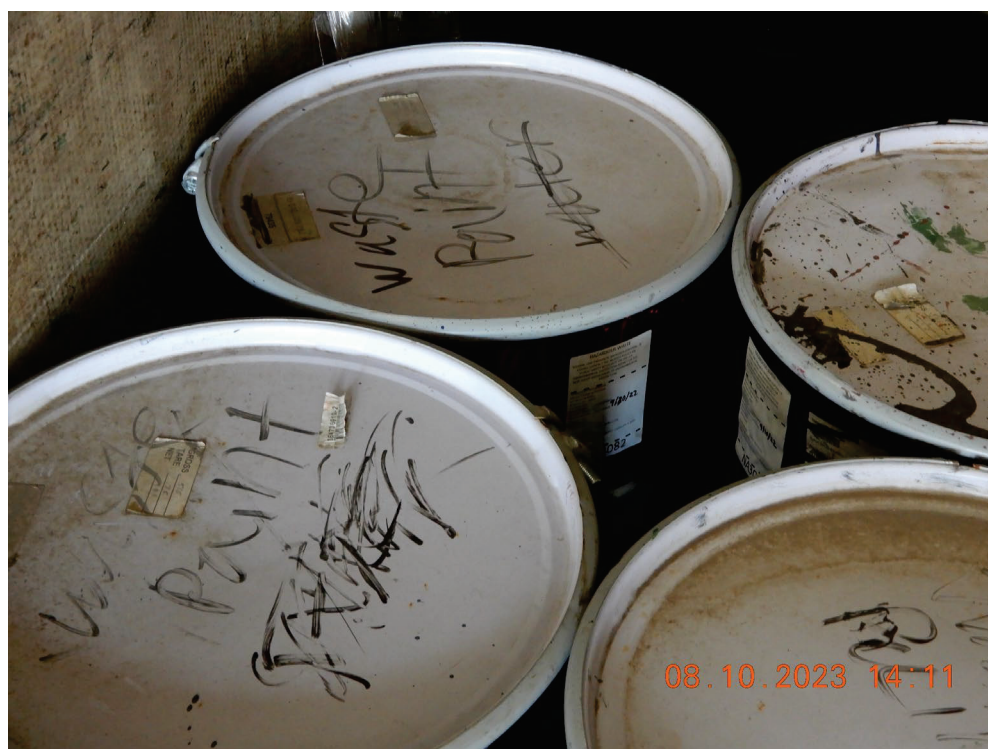
Photo 6. Drums in hazardous waste accumulation area labeled D006 hazardous waste and dated 9/16/22 and 9/20/22. (DSCN0728.JPG)
