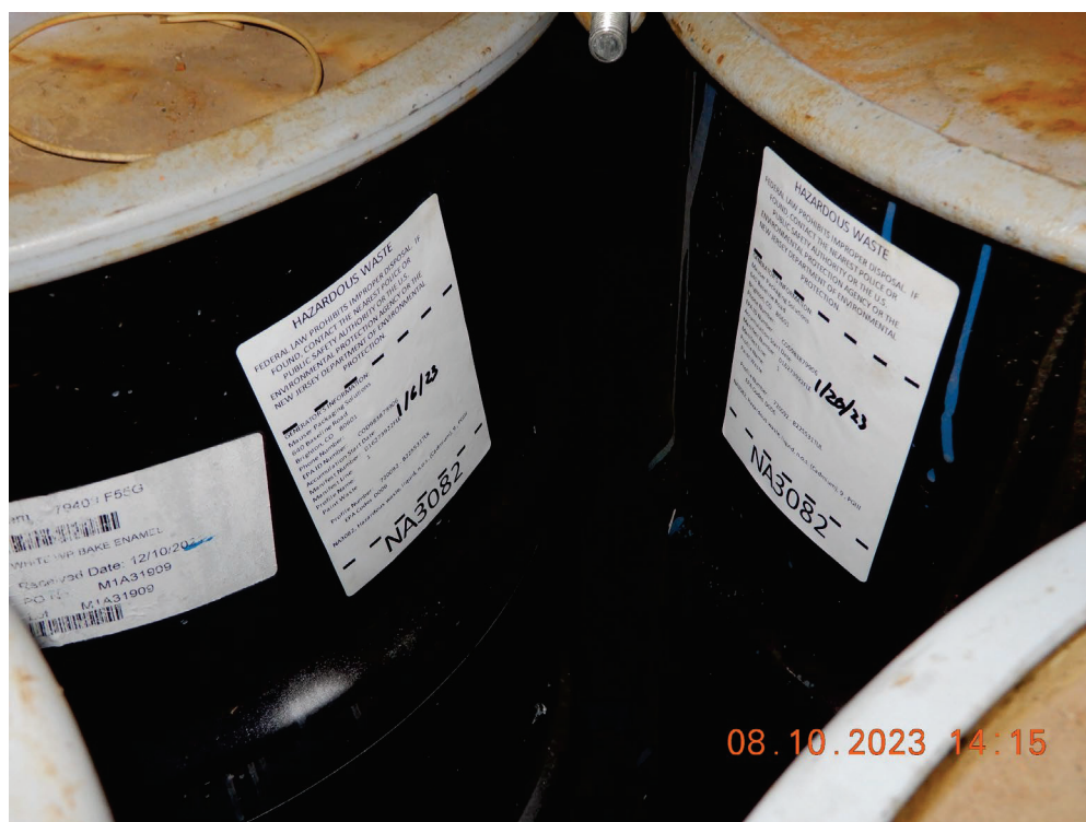
Photo 18. Clear photo for photos 16 & 17. Drums in hazardous waste accumulation area labeled D006 hazardous waste and dated 1/6/23 and 1/20/23. (DSCN0740.JPG)
