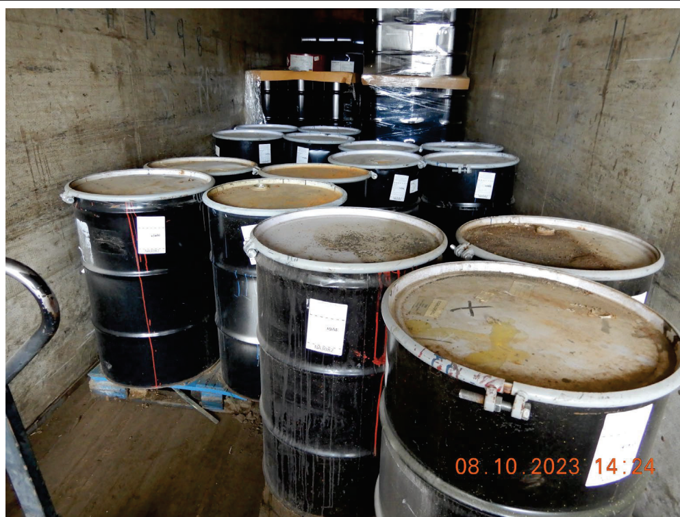
Photo 23. Overview of drums on pallets in hazardous waste accumulation area showing lack of aisle space. (DSCN0745.JPG)
