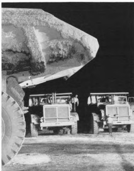
Some of the new twin-engined diesel trucks, which haul 60 tons of ore up grades as steep as 7 per cent. These trucks operate 24 hours a day. Note relative size of men.
