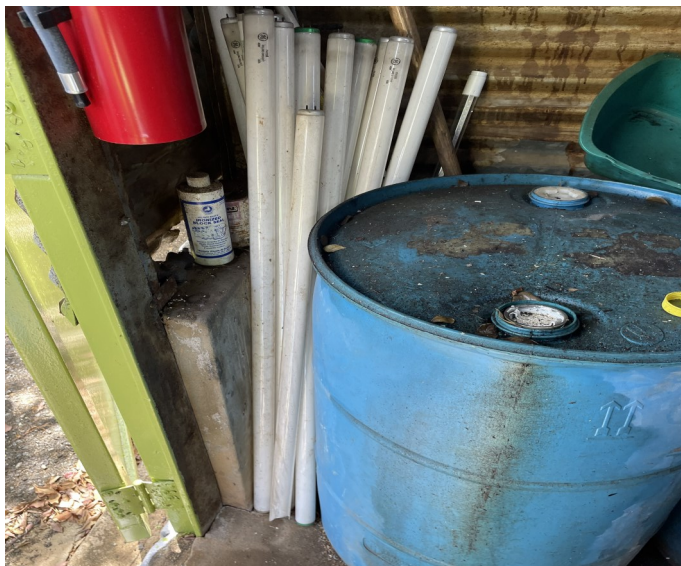
Picture 125 - UPR ALZAMORA FARM- At the Mechanic Shop there were over ten (10) 4-foot spent fluorescent lamps, on the floor without control or containment showing evidence of breakage, leakage, and damage that caused releases of mercury or other hazardous constituents to the area.
