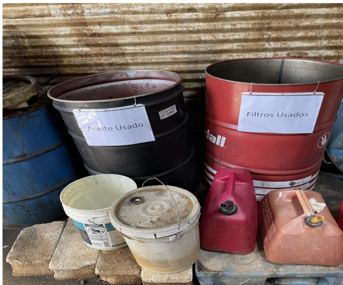
Picture 126 - UPR ALZAMORA FARM- At the Mechanic Shop there was one (1) 55-gallon red drum open on top with spent used oil filters impregnated with used oil not marked with the words, "Used Oil," (Spanish "Filtros Usados").
