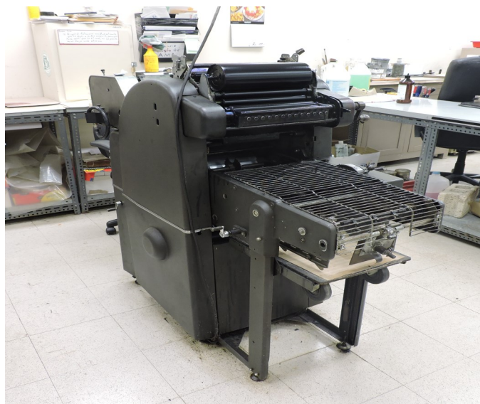
Picture 144 - UPR PRINTING DEPARTMENT - At the Printing Shop, Mr. Caban indicated that the printing used to be offset by pressing machine and that wastes used to be generated from used rags impregnated with Supreme Plate Cleaner which were collected and sent to be laundered and reused.
