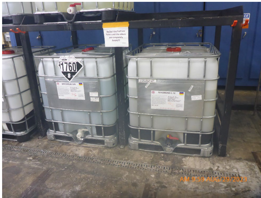
Photograph 1. Totes of starch stored without secondary containment next to a floor drain.
