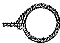
Good—Because of cutting action of eye splices on running line
