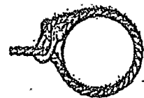
Good—No cutting action on running line
