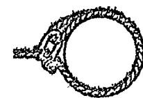
Bad—Left on running line can work loose
