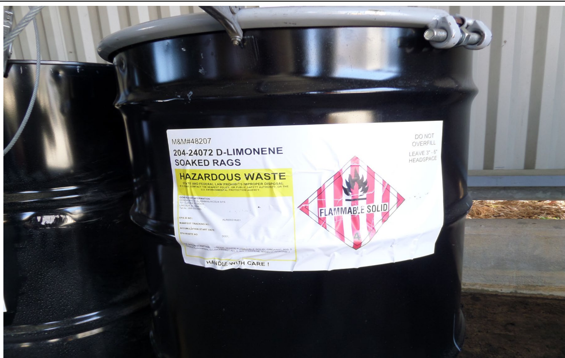
Honda Mfg. of Alabama LLC. 90-Day or Less Accumulation Area Line 2. The waste D-Limonene rags are generated at the end of the Line 2 assembly area. The waste is then transferred to this 90-Day and accumulated in a SAA. The container was not marked with a date. Photograph 3 taken at 12:45 p.m. (EST).
