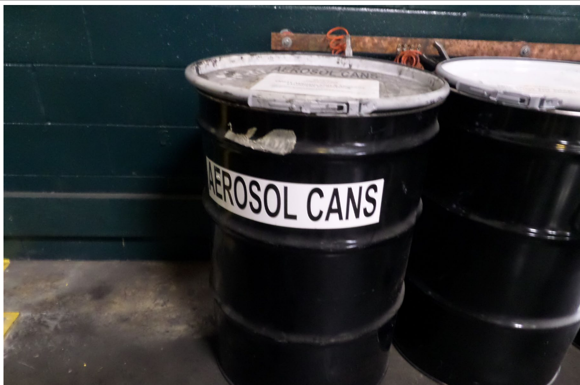
Honda Mfg. of Alabama LLC. Weld Department for Manufacturing Line 2 SAA. The inspector observed one 55-gallon metal container accumulating aerosol cans not kept closed and not marked or labeled with the words hazardous waste and not labeled with an indication of the hazard of the container contents. Photograph 4 taken at 1:06 p.m. (EST).
