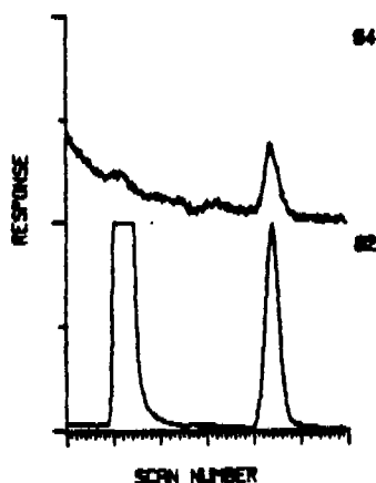
FIG. 4—Total ion current profile of Sample 3 containing 2.1 ppb VC, polymer basis (0.8 ng VC injected); retention time of VC indicated by arrow.
