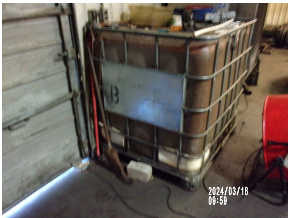
Photograph 4: Used Oil Tote Tank in the Transmission Replacement Area.
