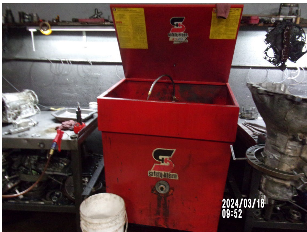
Photograph 3: Parts Cleaner in the Rebuild Area.
