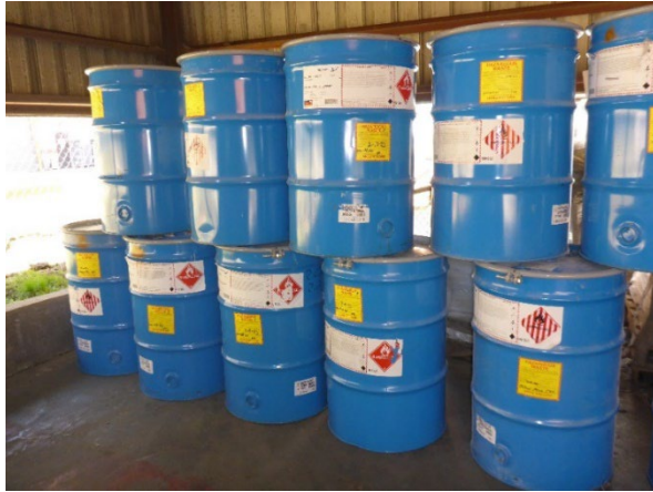
Central Accumulation Area - Photo 37: Row Four in the CAA. Drums of hazardous waste D001 flammable solids. Five drums were identified with an indication that they contained flammable liquids.
