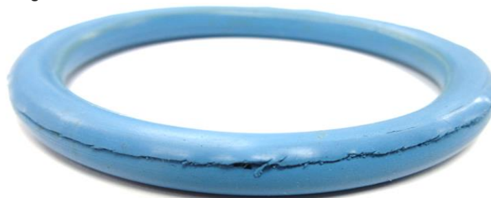
Figure 4: Swelling of a seal with low chemical resistance (e.g. non-fluorinated) used in aggressive medium (Illustration from ESBAF members)
