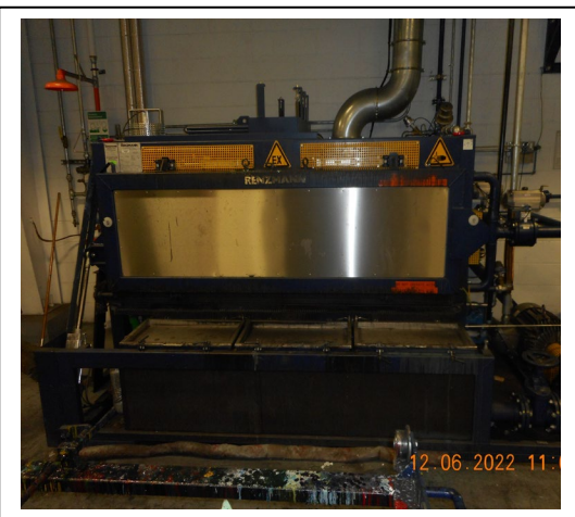
Photo #3 - Renzmann press part cleaning machine.
