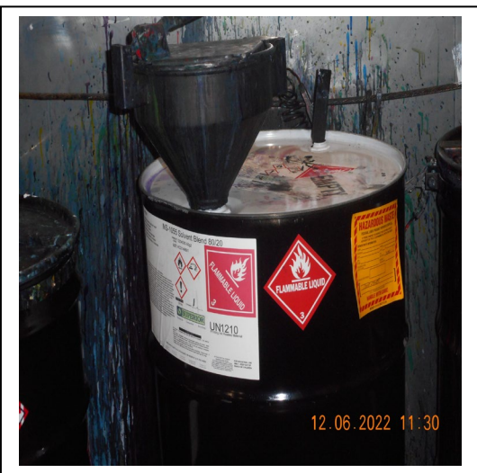
Photo #7 - open latched container of spent solvent marked "Hazardous Waste" with an indication of the hazard of the contents.
