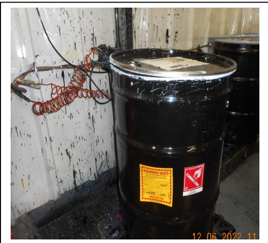
Photo #1 - open 55-gallon satellite container of waste printing near the ink storage/mixing area.
